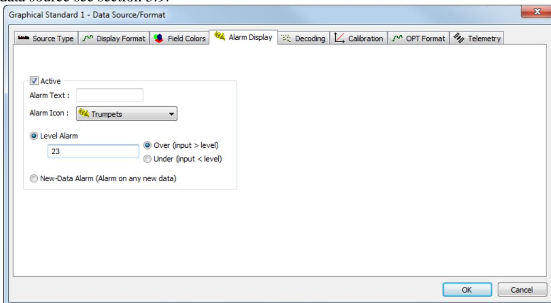
The example above shows how an alarm will be generated if, for example, the wind speed is above 23kts.
