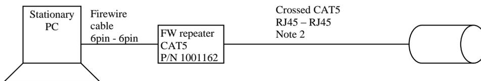
Note 2) if the original cable is attached to the capsule, then use a straight CAT5 cable and a RJ45 coupler.
