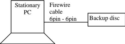
Note) if the PC is unable to power the disc then use a repeater with a mains adaptor, see below.
