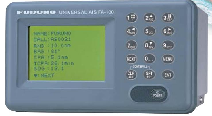
The FA-100 is a universal shipborne AIS capable of exchanging navigation and ship data between own ship and other ships or coastal stations. It complies with IMO MSC.74(69) Annex 3, A.694, ITU-R M.1371-1 and DSC ITU-R M.825. It also complies with IEC 61993-2 (Type testing standard), IEC 60945 (EMC and environmental conditions).
