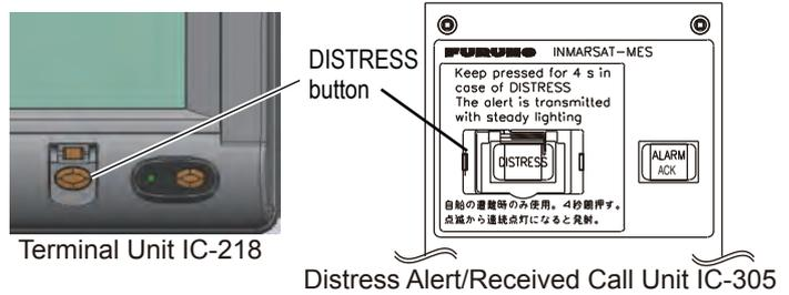
3. Press the **DISTRESS** button until (approx four seconds) the lamp in the button lights continuously. The distress alert will not be sent until the lamp in the button lights continuously and the audio alarm sounds. The message "Sending Distress Alert" appears on the screen while the distress alert is being sent.
