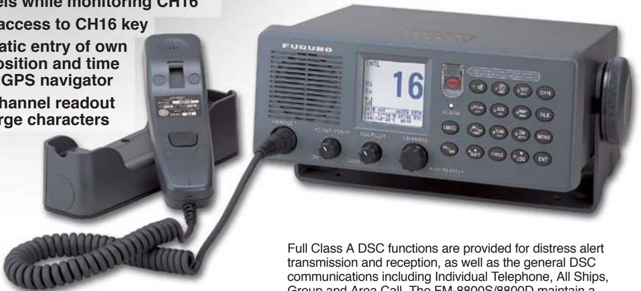
The FURUNO FM-8800S/8800D are high quality, all-in-one marine VHF radiotelephones designed to comply with the GMDSS carriage requirements for safety and general communications. All the necessary functions such as a 25 W VHF radiotelephone, a Class A DSC modem and a CH 70 Watch Receiver are incorporated into the compact transceiver unit.
