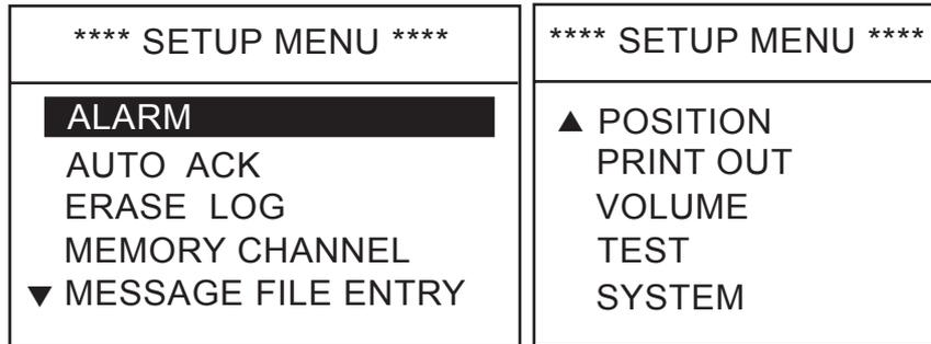
2. Rotate the **CH** knob (or press up / down arrow key) to choose SYSTEM from page 2 of the menu and press the **ENT** key. The following window appears.
