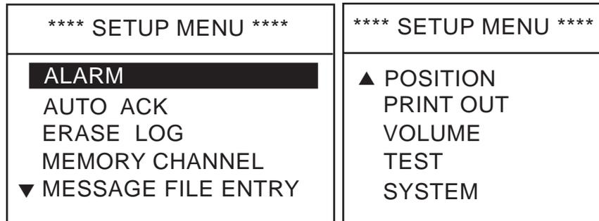
2. Rotate the **CH** knob (or press up / down arrow key) to choose **SYSTEM** from page 2 of the menu and press the **ENT** key. The following window appears. The self ID is displayed on the first line.
