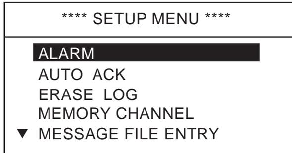
2. Rotate the **CH** knob (or press up / down arrow key) to choose MESSAGE FILE ENTRY and press the **ENT** key.
