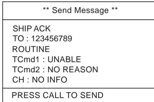
6. Press the **CALL** key more than three seconds to transmit the ACK BQ. The display changes to the standby display.
