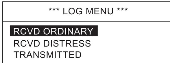
2. Rotate the **CH** knob to choose RCVD ORDINARY, RCVD DISTRESS or TRANSMITTED as appropriate and press the **ENT** key. For example, choose RCVD ORDINARY or TRANSMITTED.
