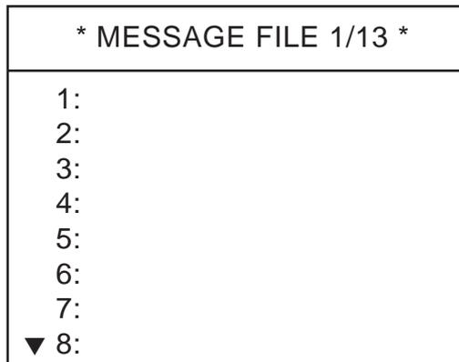
3. Rotate the **CH** knob to choose a vacant number and press the **ENT** key. The following selection window appears.
