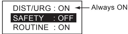
2. Rotate the **CH** knob (or press up / down arrow key) to choose an appropriate option. Alarm is output to external device.
