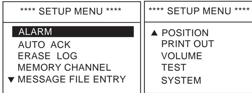
2. Rotate the **CH** knob to choose **SYSTEM** and press the **ENT** key. The following selection window appears.
