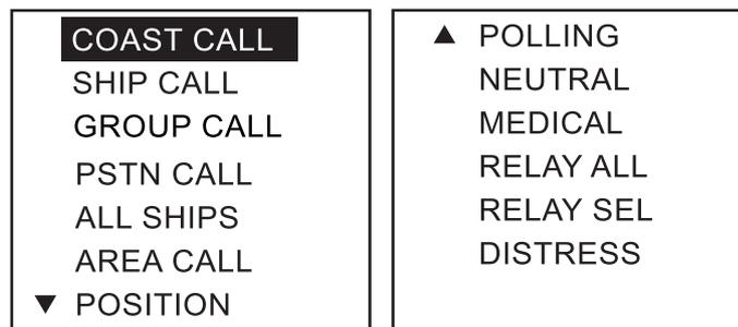
3. Rotate the **CH** knob (or press up / down arrow key) to choose ALL SHIPS and press the **ENT** key.
