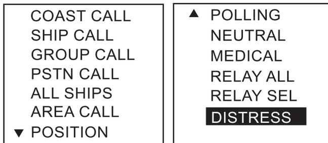
3. Rotate the CH knob (or press up / down arrow key) to choose DISTRESS. Press the **ENT** key.
