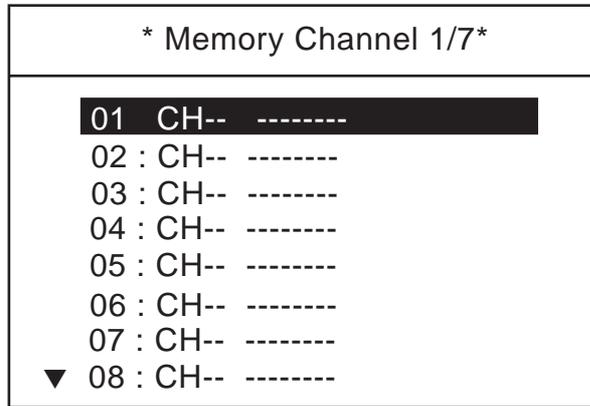
3. Rotate the **CH** knob (or press up / down arrow key) to choose a vacant CH number and press the **ENT** key.
