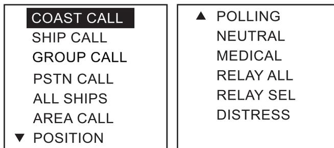
3. Rotate the **CH** knob (or press up / down arrow key) to choose COAST CALL or SHIP CALL and press the **ENT** key.
