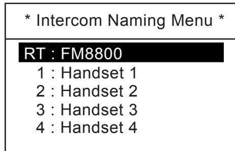
4. Rotate the **CH** knob (or press up / down arrow key) to choose a handset number and press the **ENT** key.
