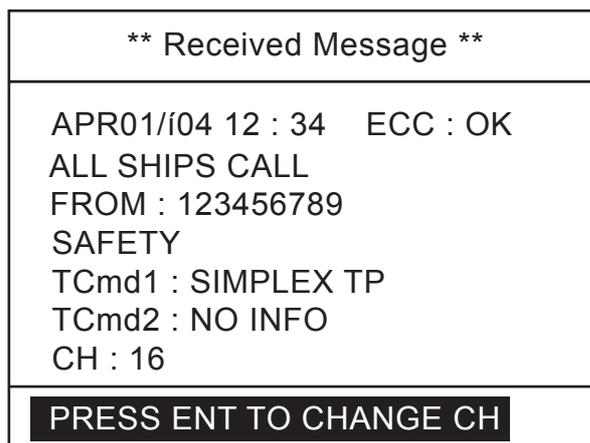
3. Press the **ENT** key. The display changes to the standby display, indicating channel specified, and you can watch the contents of the message.
