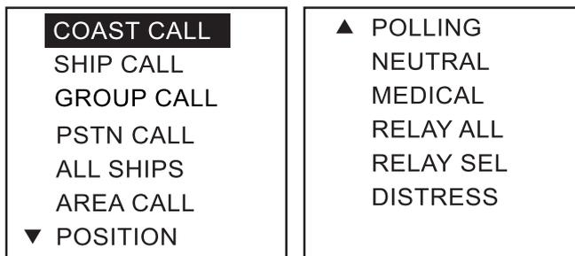
3. Rotate the **CH** knob (or press up / down arrow key) to choose PSTN CALL and press the **ENT** key.
