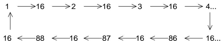
To start scanning, press the **SHIFT** and **8 SCAN** in that order. When the receiver finds a signal, scanning is stopped on that channel and starts dual watch on it and CH16.
