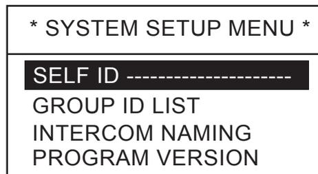
3. Rotate the **CH** knob (or press up / down arrow key) to choose INTERCOM NAMING and press the **ENT** key. The following window appears.
