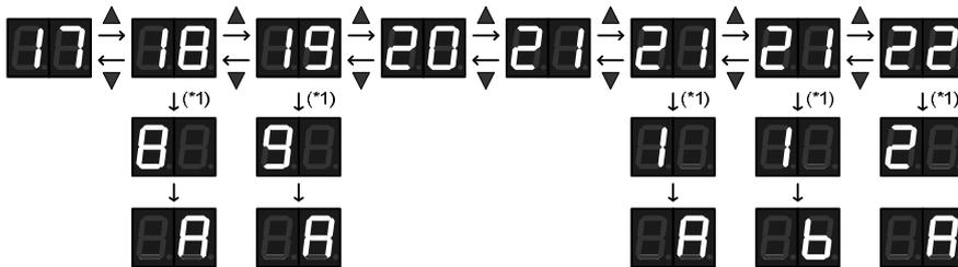
\*1) If left the ▲ or ▼ key on the channel, the digits of the channel start scrolling. For more details, see 7.Display below.
