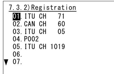
2. Move the cursor to the desired list number and press ENT using the jog dial, or press the memory channel number (two digits) by numeric keys directly. Then select a channel type.
