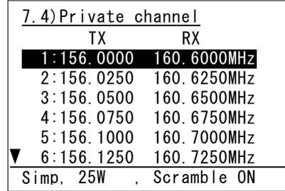
2. Move the cursor to the desired channel number and press ENT using the jog dial, or press the private channel number (three digits) by numeric keys directly.
