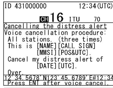
5. When the cancelling procedure is completed, displays the operating screen as shown at right and finishes the distress mode.
