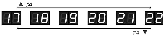
\*2) While holding down, channel number is increasing at the same interval of time (0.5sec). Additionally, if left the ▲ or ▼ key, the digits of the channel start scrolling as mentioned above.
