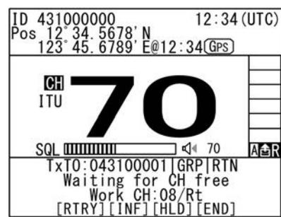
5. After sending the message, the working channel is set and the DSC calling procedure is finished.
