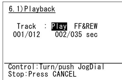
2. After finishing the playback of the latest track, the cursor automatically moves to **Track** and the function is stopped.
