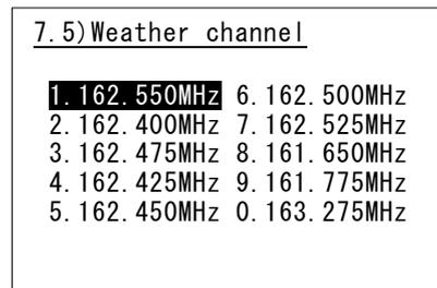
2. Move the cursor to the desired line and press ENT using the jog dial, or press a numeric key directly.
