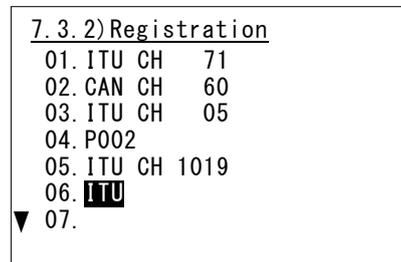
3. Press ENT after selecting a channel type. Then input the channel number using the jog dial or numeric keys.
