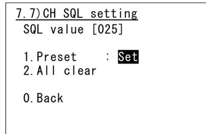
**4.** To complete the squelch setting for the channel, select "Set" and press ENT.
