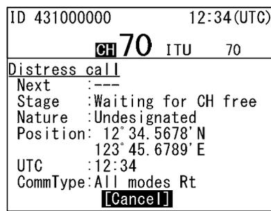
4. After sending the distress alert, wait for the acknowledgement in the condition of the activated distress transmission procedure.
