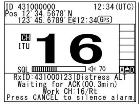
**Note** Even If there is no active procedure as above, when the menu "9.5.8 Auto CH change" is OFF, the channel is not automatically changed to CH16. In this case, after pressing the **CANCEL** key to stop the alarm, select the "Accept" on the popup screen to set the CH16 and skip to step 3.
