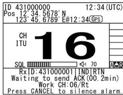
2. Press the **CANCEL** key to stop the alarm and display the screen at right.
