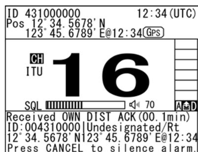
4. After receiving acknowledgement, lift the handset and request rescue using CH16 of the radiotelephone.
