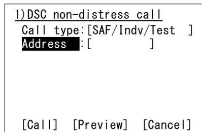
2. Press ENT on the Call to start sending the safety test call.
