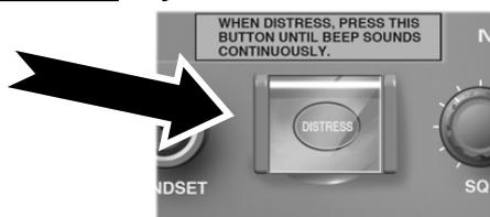
2. Press and hold the **DISTRESS** key for 4 seconds. (See the note below.)
