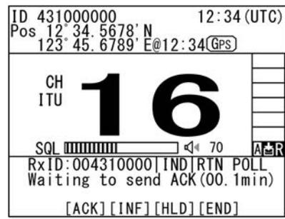
Additionally note that if it is received while the 9.5.1.3 Polling call of the Automatic ACK menu is set to ON, and there is no active procedure, this call can be acknowledged automatically.
