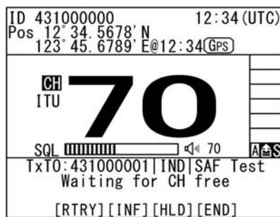
3. When the acknowledgement is received, the ALM lamp blinks and the alarm starts sounding. After silencing it with **CANCEL** key, the screen becomes as shown at right.
