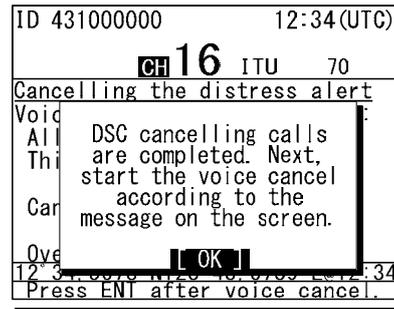
4. According to the guidance on the screen, broadcast to cancel the distress alert.
