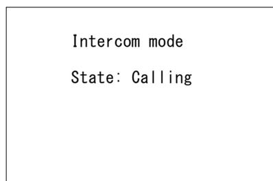
**Note** - When starting the call, if the handset of the recipient is left off-hook, the call is not started and the screen at right is displayed. Then press ENT to return to the step 1.
