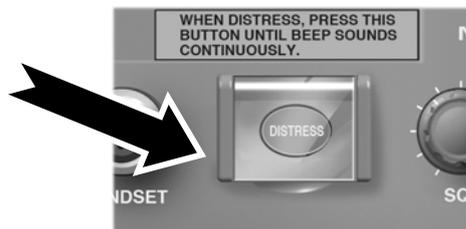
2. Press and hold the **DISTRESS** key for 4 seconds until the countdown is completed.
