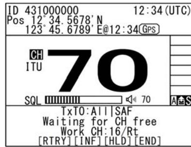
3. After sending the message, the working channel is set and the DSC calling procedure is finished.
