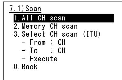
2. Move the cursor to the desired item and press ENT using the jog dial, or press the item number by a numeric key directly.
