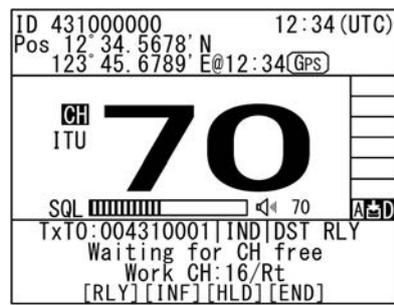
5. When receiving the acknowledgement from the coast station, the screen shows as shown at right.
