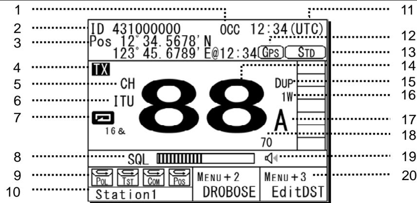
1. Occupied mark indicates when the other controller has the access rights.
