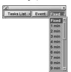
Select the required vector length (see document NAVI-SAILOR 4000/4100 ECDIS (v. 2.00.009). FUNCTIONAL DESCRIPTION, Chapter 3, section Own Ship Motion Data, paragraph Own Ship Motion Vectors) from the list, which will open up and press the left trackball/mouse button.
