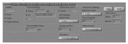
In AutoZoom Settings group from the drop-dawn list, select the maximum scale as the ship is passing the current WPT on "Dual" panel. In Time of update input window set the DTW analysis interval.
