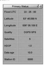
"Primary Status" display is used for presenting the following data from EPFS, which used as primary positioning system:
