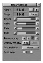
In "Radar Settings" display which will open up, set the range scale. To do this, use the buttons to the right of Range input window.
