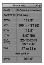
"Route Data" display is intended for the display of data as the ship is proceeding along the route to the next waypoint (see document NAVI-SAILOR 4000/4100 ECDIS (v. 2.00.009). FUNCTIONAL DESCRIPTION, Chapter 5, section Route Monitoring, paragraph Sailing Along the Route). The display contains the following data:
