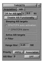
In the input line to the right of the DR for AIS tgts button, set the minimum speed of AIS targets for the DR mode.
