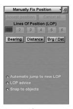
"Manually Fix Position" display is intended for constructing the ship line of position (LOP) by measuring bearing and/or range to one or more visible objects whose coordinates are known in advance (or the object can be uniquely identified on the chart).
