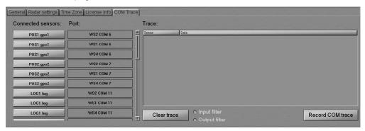
This page is intended for displaying and recording of the IEC 61162-1, 61993-2, and proprietary (e.g. for ES4/ES3) formats and similar text messages/sentences provided to the NS 4000 MFD from the external sensors and displaying of the sentences transmitted by the NS 4000 MFD to the external devices.
