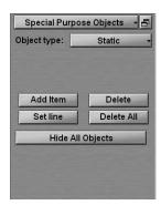
This NS 4000 MFD functionality enables special purpose objects (SPO), mobile and fixed, with certain features to be created and referenced to an electronic chart with the purpose of their further monitoring and obtaining of auxiliary information.
