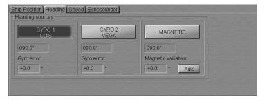
"Heading" page is designed for selection of heading source. "Heading" page shows all the connected heading sensors.
