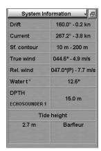
In DPTH row it is displayed value of water depth under the keel (from the sounder data).
