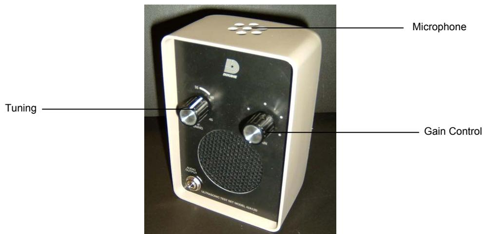
Figure 19-1 - Dukane 42A12D Beacon Test Set
