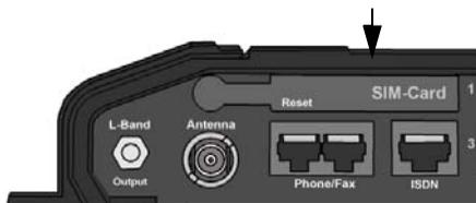
2. Insert the SIM card into the SIM slot.
