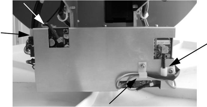
3. Unscrew the four finger nuts on the back of the HPA and gently remove the HPA.
