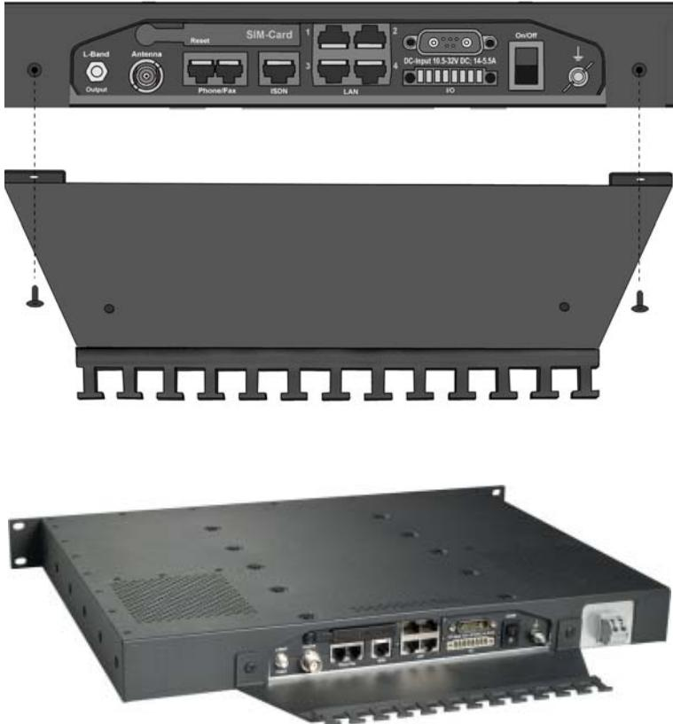
3. Install the terminal as described in *Installing the terminal* on page 46.
