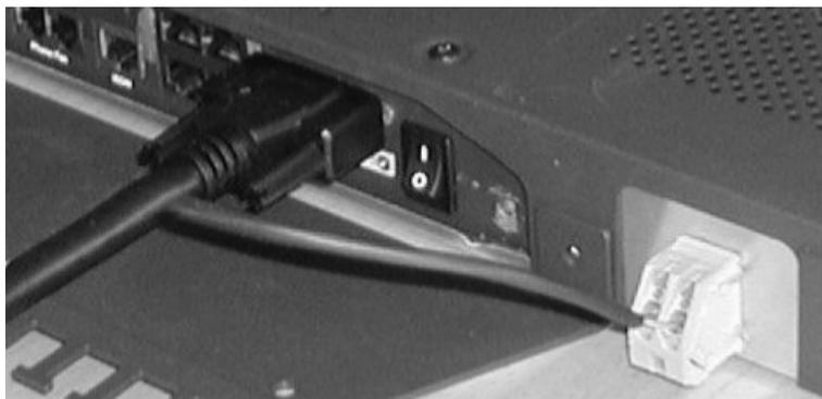
If you want to use the power switch on the front of the terminal to switch the terminal on and off, connect the remote on/off pins in the DC connector to the terminal block in the connector panel as follows:
