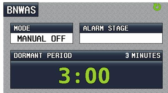
2) **MANUAL ON**: BNW-50 operates constantly. And it shows " **MANUAL ON** " for MODE, on the operation screen.
