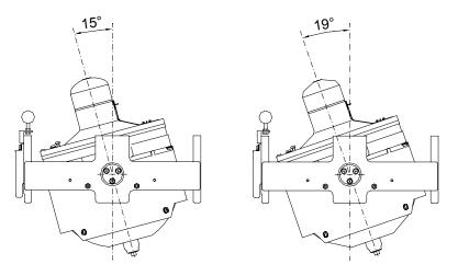
Max and min tilt angle for GC80 std system
