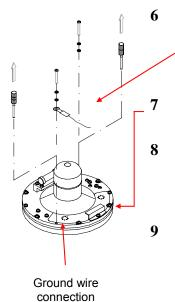
Replace the assembly jigs with the two remaining screws. Locate the ground wire on one of the screws as shown on the figure.
