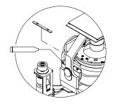
4 Lift the lid from the damper oil case, and fill the container with the supplied damper oil. The oil has high viscosity, and care should be taken when pouring the damper oil into the container to avoid spill. Reinstall the lid on the damper oil case.
