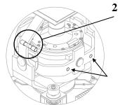
Locate the reference level tool on the horizontal ring, and check that the level bubble is within +/-10 minutes from the center. Each division equals 2 minutes.
