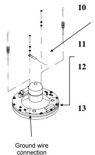
Replace the assembly jigs with the two remaining screws after placing the ground wire as shown on the figure.
