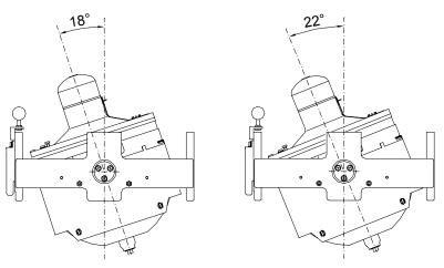
Max and min tilt angle for GC85 High Speed system
