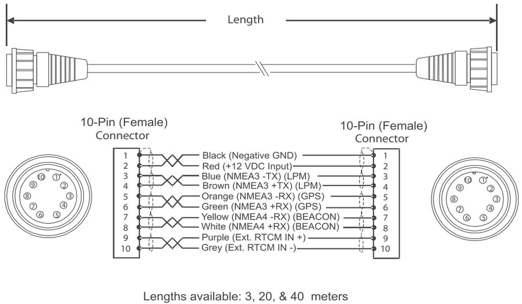
Figure 5.17 Double-Ended Antenna Cable Diagram
