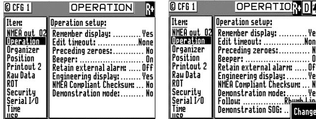
In the **CFG** *Operation* screen, activate the *Demonstration Mode* by selecting *Yes*.
