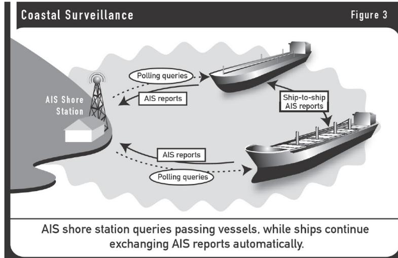
Coastal nations may use AIS to monitor the movement of hazardous cargoes and control commercial fishing operations in their territorial waters. AIS data can be logged automatically for playback in investigating an accident, oil spill or other event. AIS is also a useful tool in search and rescue (SAR) operations, allowing SAR coordinators to monitor the movements of all surface ships, aircraft and helicopters involved in the rescue effort.
