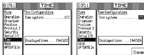
*Time System:* Sets the time to *UTC* (default) or *Local*. When *Local* is selected, several parameters associated with local time are displayed.
