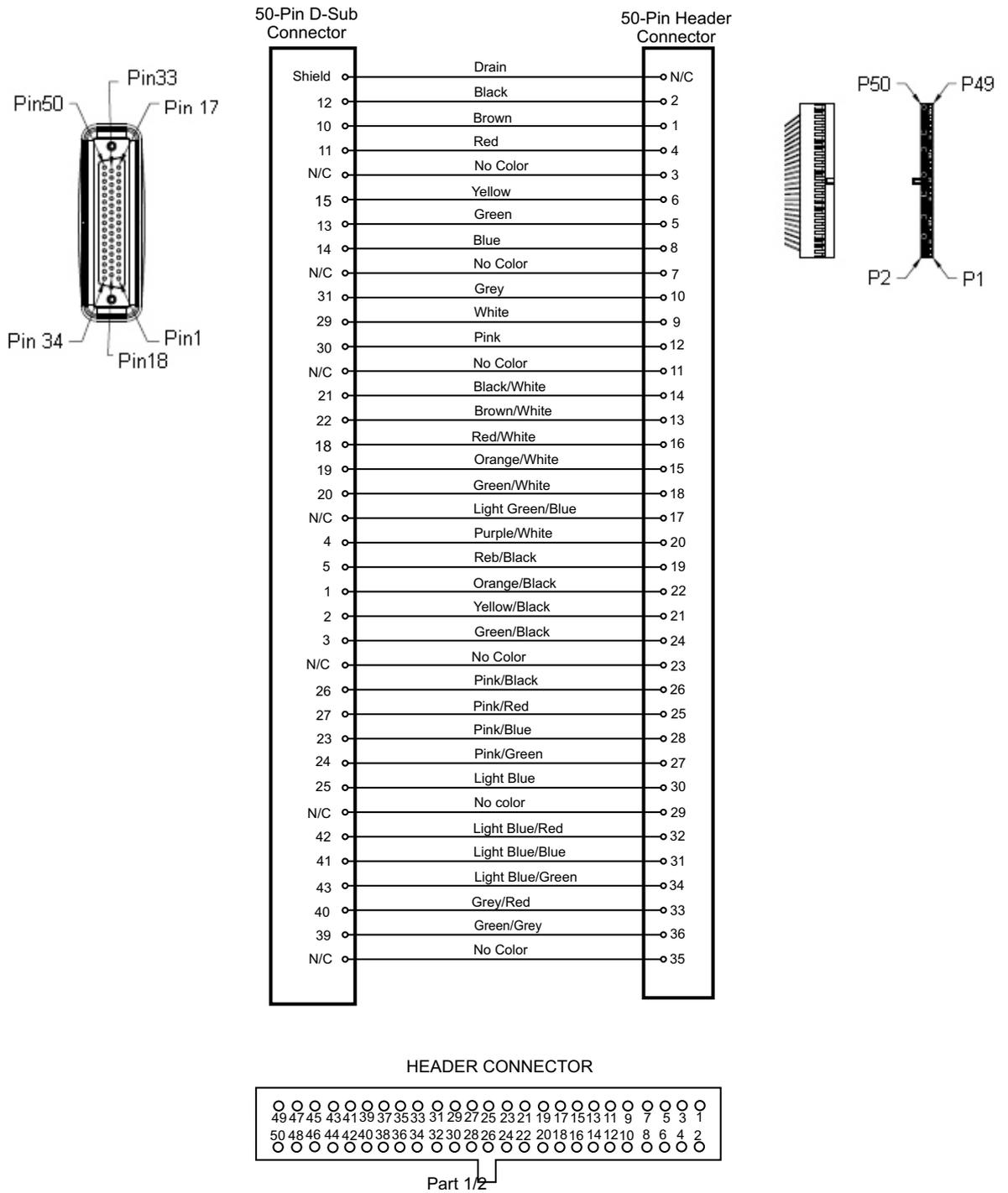
Figure E-5: 50-Pin Cable Assembly (part A)
