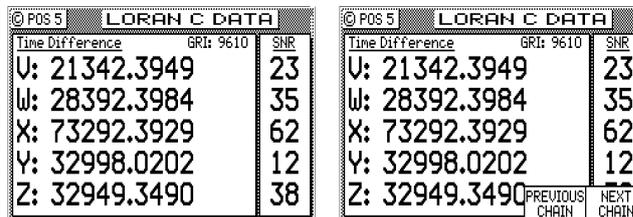
The POS 5 screen displays the Station GRI, Time Difference (TD), Warning status (CYCLE, BLINK), and Signal-to-Noise (SNR) data for different slave stations of a particular Loran-C chain being used.
