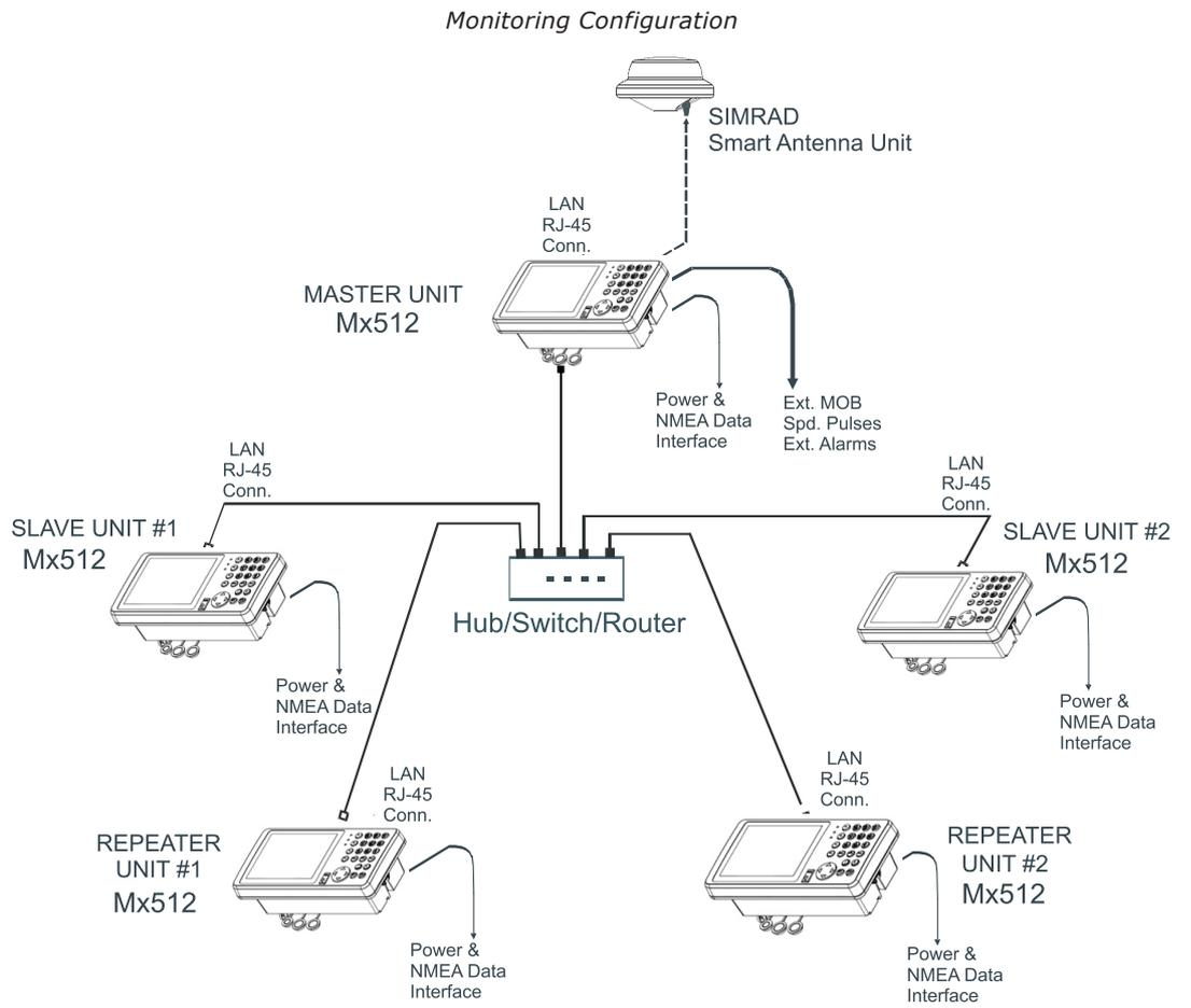
Figure 5.33 - Multiple Unit Control Configuration
