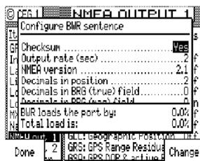
Highlight the *Details* softkey then press **ENT** to view the characteristics for the NMEA record you select. If you notice that the top of some text is cut off by the *Capacity Needed* window, this indicates that there are more selections available than can fit in the window. Use the cursor key to scroll down the list. Each record is controlled separately. Generally speaking, the following controls are available to you for most or all of the records:
