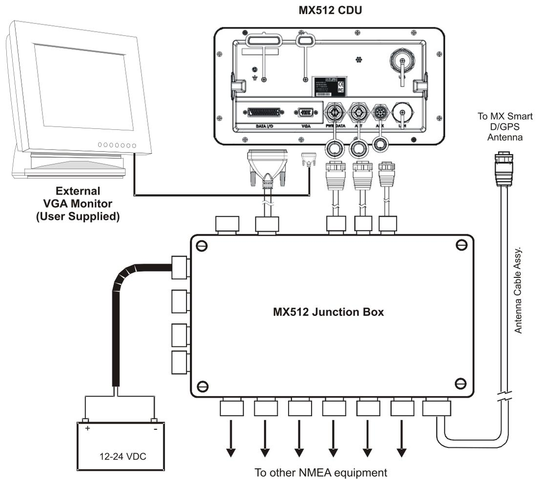
Figure 5.25 - MX512 Junction Box Assembly
