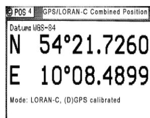
The *POS 4* screen displays the *GPS/LORAN-C combined position* and navigation modes received from the *\$PMVX1* message (which is based on (D)GPS if GPS is available, and based on (D)GPS calibrated LORAN-C position if GPS is not available) from the LORAN-C receiver. The *\$PMVX1* message is formatted just like the NMEA GGA message, except that its GPS quality indicator ranges from 0-5. The GPS quality indicator is displayed as a navigation mode on the *POS 4* screen.
