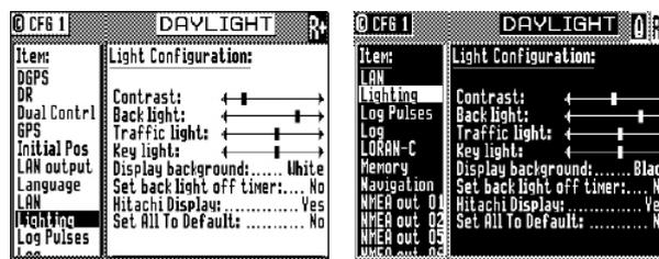
*Contrast*- Controls the viewing angle of the display
