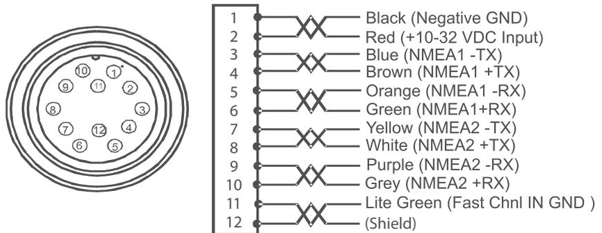
Figure 5.26 - 12-Pin Power/Data Cable Assembly Diagram
