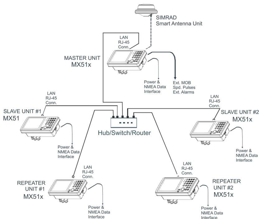
The interface among the units takes place over a high speed (100 Mbps) data link. The master unit must be connected to the antenna. The master unit receives the NMEA signals from an MX antenna and pass it along to the slave and repeater units at a one second rate. Due to the high speed data link, there is virtually no visible position delay among the units.
