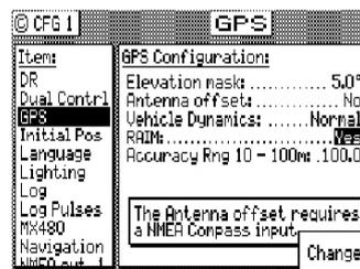
The *RAIM* menu is available only in MX51x models where the RAIM feature is enabled. For more detailed information about RAIM, please refer to Page 67 of this manual. Standard MX51x CDU will only show the Elevation mask and Antenna offset menu items.
