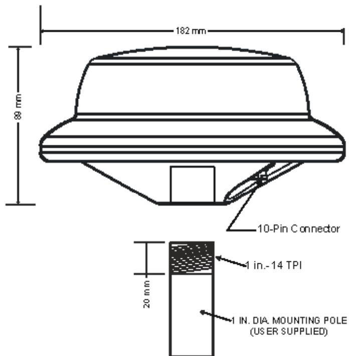
**Figure 5.8 - Standard Smart Antenna Dimensions and Mounting Specifications**
