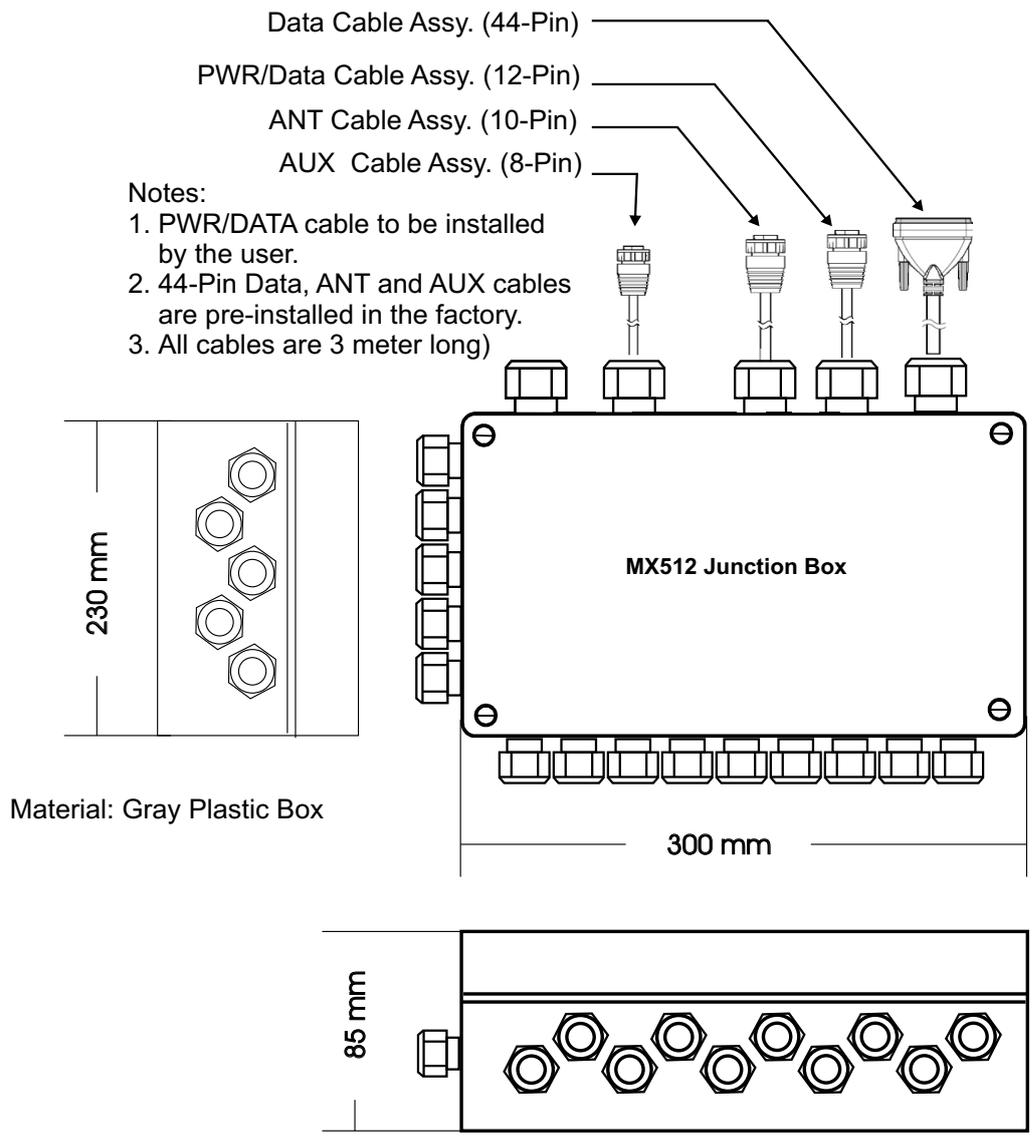
**Figure 5.11 - MX512 Junction Box Dimensions**
