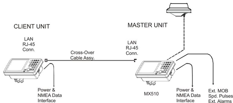
The hardware interface is accomplished by connecting the RJ-45 connectors of the MX51x units using a crossover (null) LAN cable (for two units) or CAT5 Ethernet cables with an Ethernet switch (for more than two units). You can purchase a pre-made LAN crossover cable or CAT5 Ethernet cable assembly from MX Marine dealers or you can make it up yourself using the diagram below.
