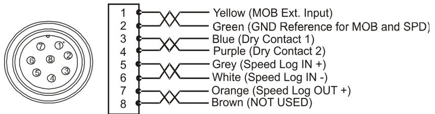
Figure 5.16 Auxiliary Cable Diagram
