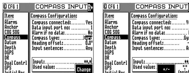
Specify the input NMEA 0183 record for the *Input Sentence*. HDT, HDG, HDM, HCC, HCD, VHW, or Any.
