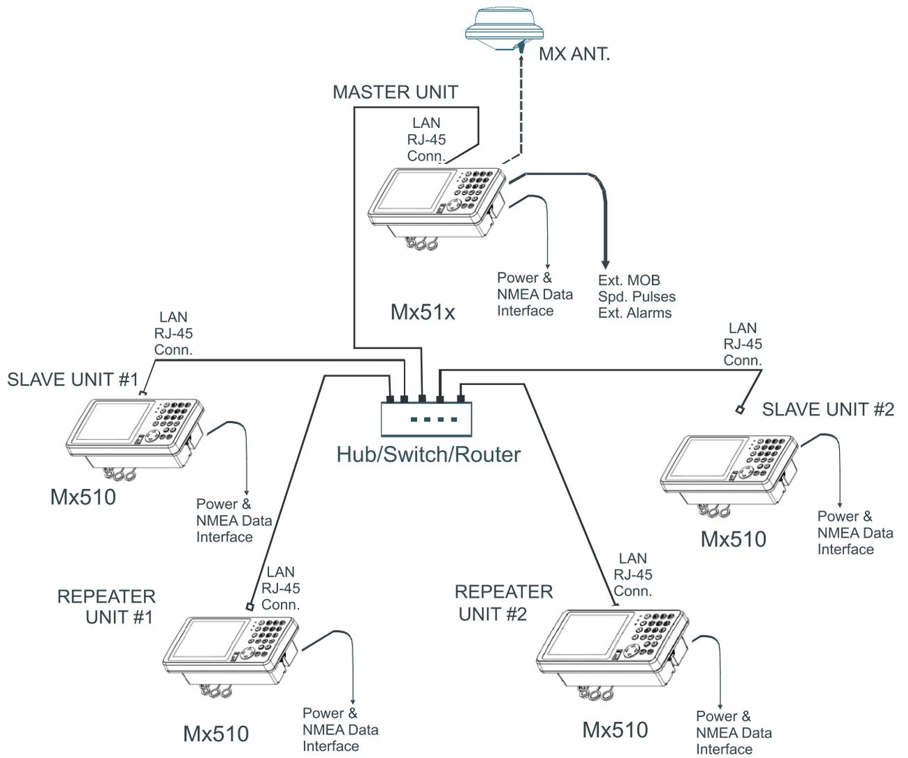
Figure 5.23 Multiple Control Configuration
