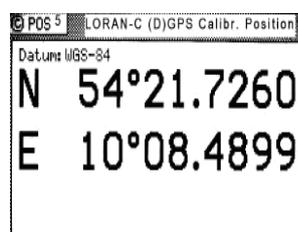
The POS 5 screen displays the (D)GPS calibrated LORAN-C position received from the GLL message from the LORAN-C receiver.
