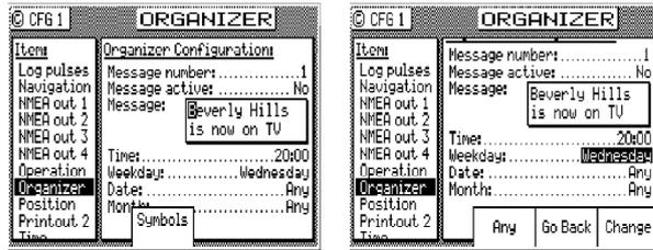
The setup is straight forward. Use the *Change* softkey to increment forward through the available choices. Use the *Go Back* softkey to increment backward through the available choices. You can also use the left and right cursor keys to accomplish these same operations. Enter text the same as you do for the waypoints and routes. Use the numeric key pad to enter the appropriate time. Don't forget to set *Message Active* to *Yes* when you are finished editing, to enable the alarm.
