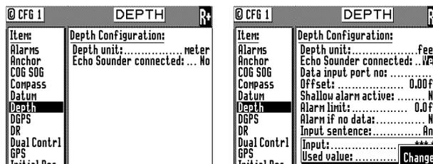
Press the **EDIT** key and move the cursor to the *Echo Sounder Connected* line. Press the ENT key to *Change* softkey to activate the input data options described below:
