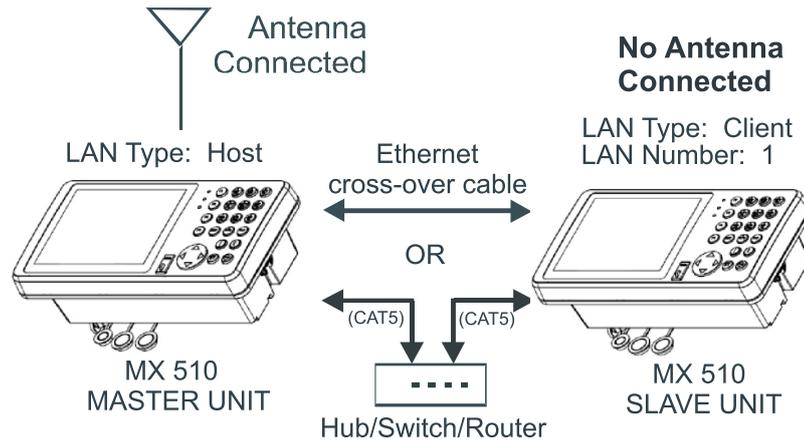
The interface between the two units takes place over a high speed (100 Mbps) data link. The master unit must be connected to the antenna. The master unit receives the NMEA signals from the smart antenna and pass it along to the slave unit. Due to the high speed data link, there is virtually no visible position delay between the two units.
