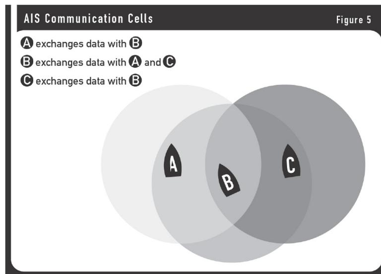
Each ship broadcasts its AIS messages and receives messages from all ships within VHF radio range. The area in which AIS messages can be received is called the ship's "cell". Each ship is in this way in the center of its own communication cell.
