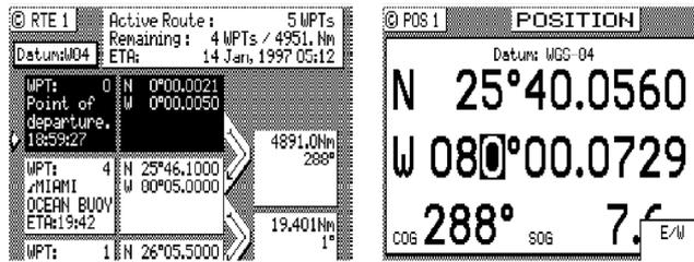
Before you adjust your position, set your *WPT Pass Criterion* to *Distance* in the *CFG1 Navigation* screen. To adjust your position, pick a point near your first waypoint. A distance of 1 or 2 miles from the first waypoint is good to start with. Go to the **POS1** screen and press **EDIT**.
