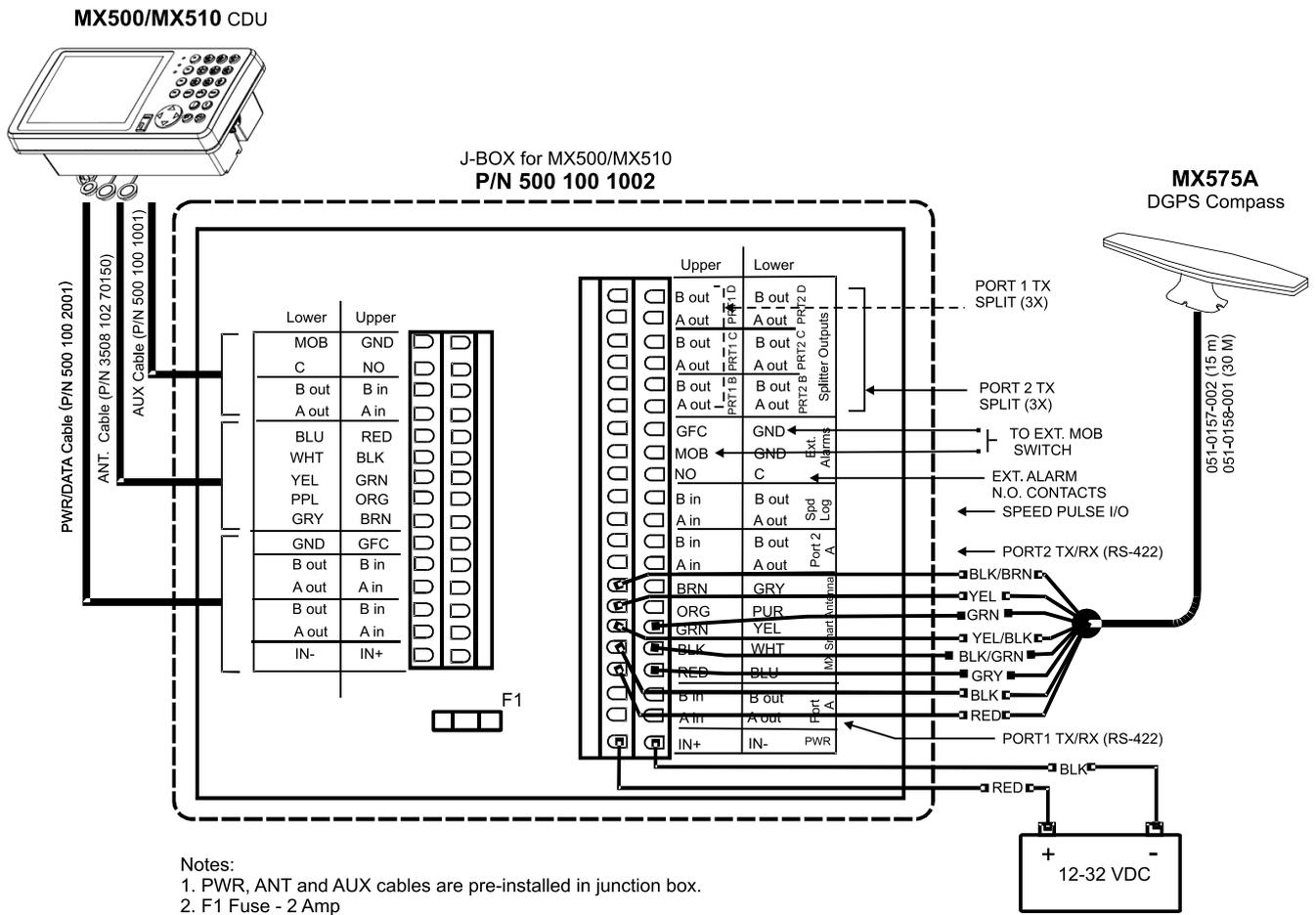
Figure 5.19 MX510 to MX575A GPS Compass Wiring Diagram
