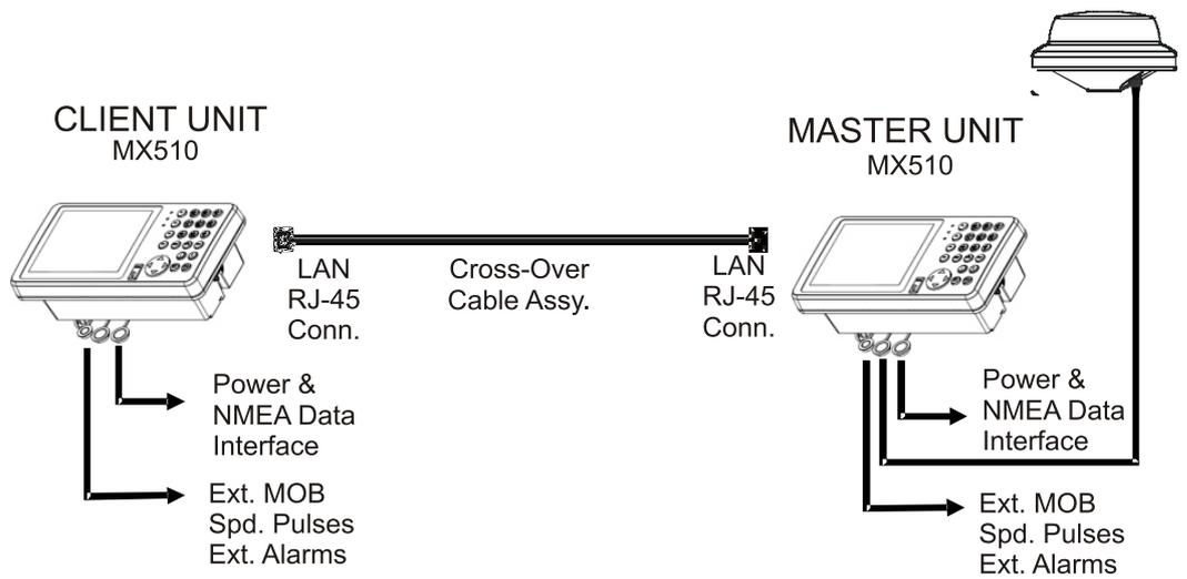
Figure 5.21 MX510 Dual-Control Configuration
