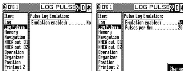
Activate the output by selecting *Yes* to *Emulation Enable* and set the pulse rate based on the device that you are connecting to.
