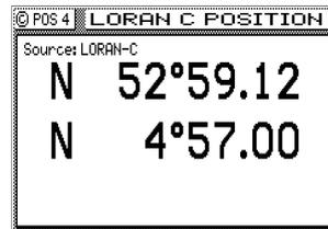
The POS 4 screen displays the geographical coordinates of the Loran-C position in the form – degrees, minutes, and hundredths of a minute.
