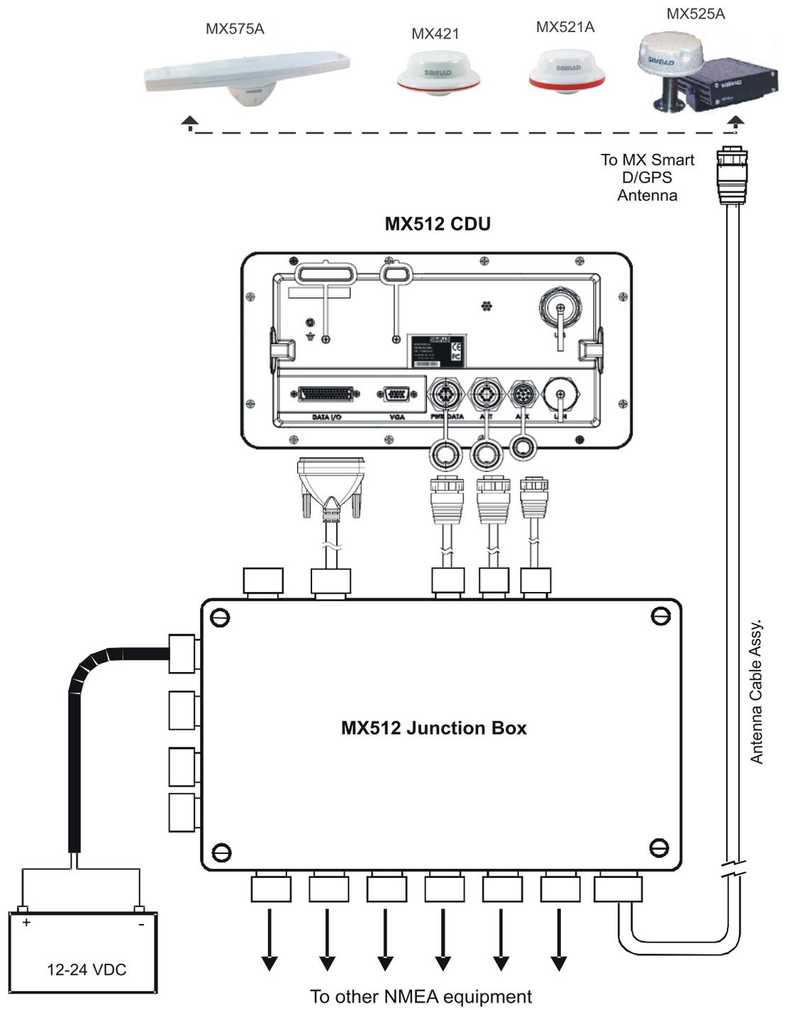
Figure 5.24 - MX512 Basic System Configuration
