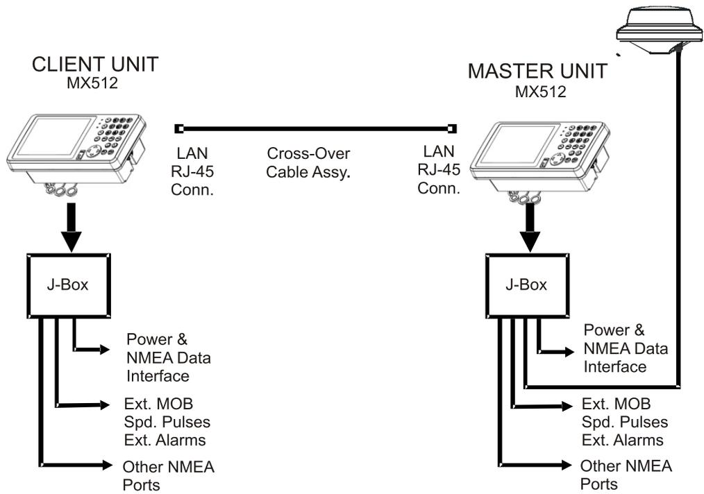
Figure 5.31 - MX512 Dual Control Configuration
