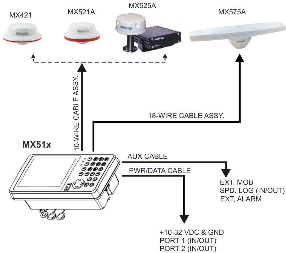
Figure 5.12 MX 510 Basic System Configuration
