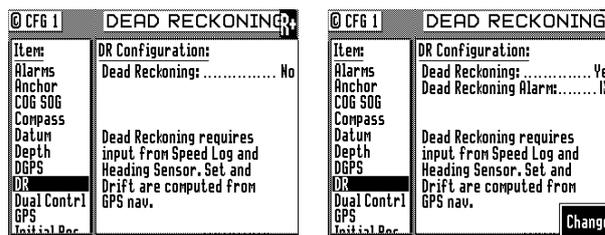
To set the DR to 'Yes', scroll down to DR menu then press the **EDIT** key. Press the **ENT** key to activate the 'Change' softkey. Press the **EDIT** key again to exit the edit mode.
