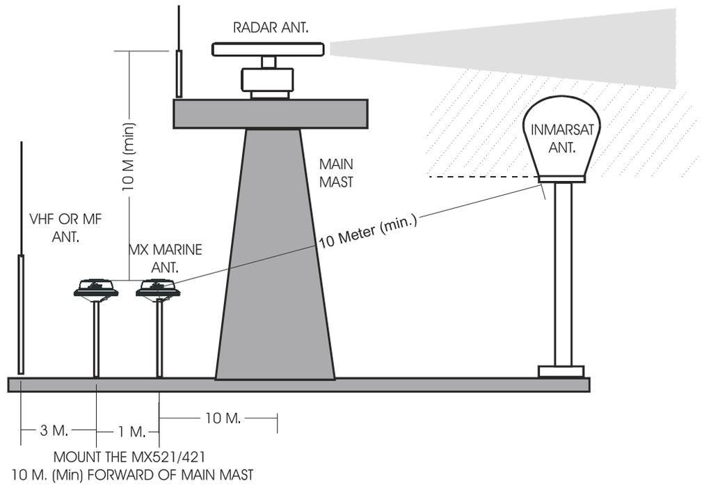
**Figure 5.9 - Antenna Location Diagram**
