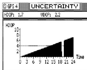
The small 1 hour gap in the bar graph represents the 24th hour. The gap is provided to ease the readability of the bar graph for the present time. The dashed line extending horizontally from the 4 represents the current *HDOP Limit Alarm*, which is set in **CFG Position**. The current HDOP and VDOP values are given in the upper window.
