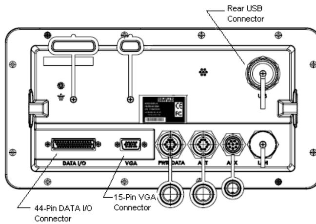
**Figure 5.4 - MX512 Rear Connector Configuration**
