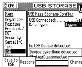
To implement this feature, plug your USB device into the USB port of the MX51x CDU first, and change *USB Connected* to *Yes*. Allow a few moments for the CDU to read and detect your USB device. Ensure that status displays *Connected* before continuing.
