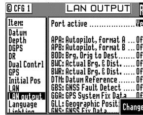
This feature can be used to integrate the MX 510 to an Integrated Bridge System by connecting the CDU to a PC-based IBS system using LAN (RJ45).
