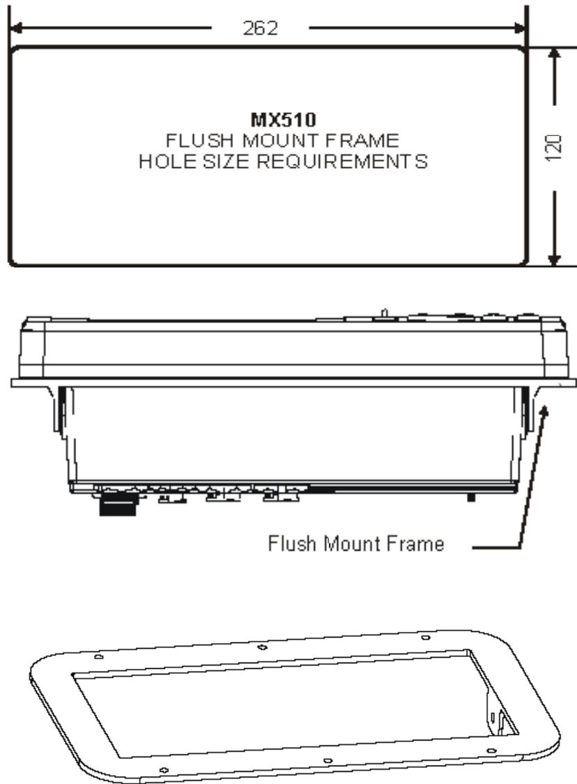
*Figure 5.6 - Optional Flush Mounting Frame*
