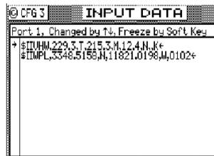
Press the up or down cursor key until the proper input port number is selected.
