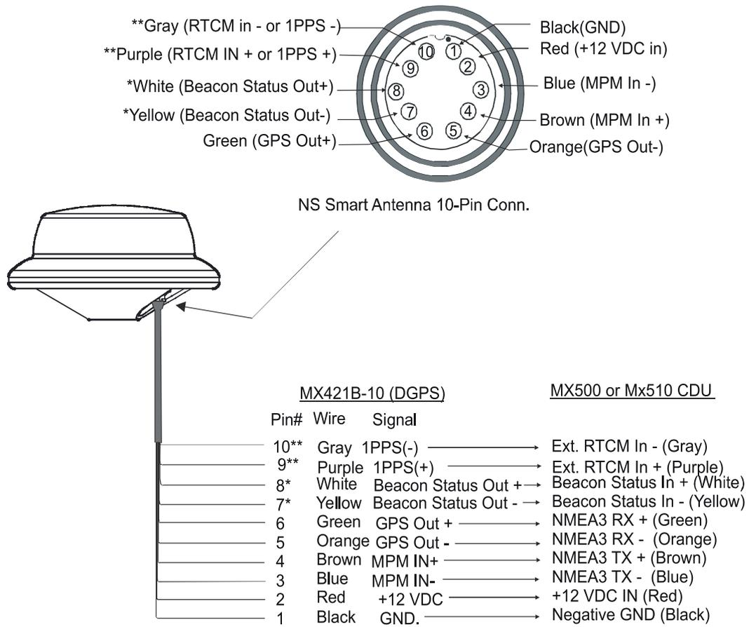
\*Not connected in MX421 (GPS only) Antenna model
