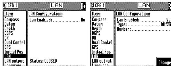
To activate *LAN*, press the **EDIT** key and press the ENT key to activate the *Change* softkey to change *LAN Enabled* to *Yes*. Use the *Change* softkey to modify the options described below:
