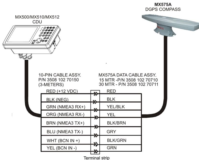
Figure 5.30 - MX51x to MX575 Antenna Wiring Interface
