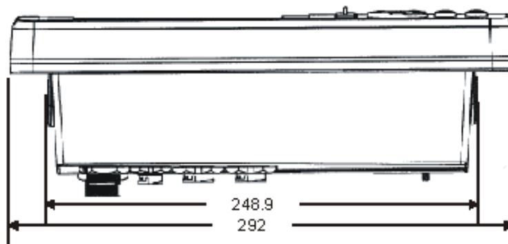
**Figure 5.2 - MX510/MX512 Display Console (Top View )**
