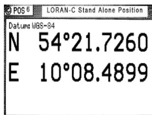
The POS 6 screen displays the stand-alone (uncorrected) LORAN-C position received from the RMA message from the LORAN-C receiver.
