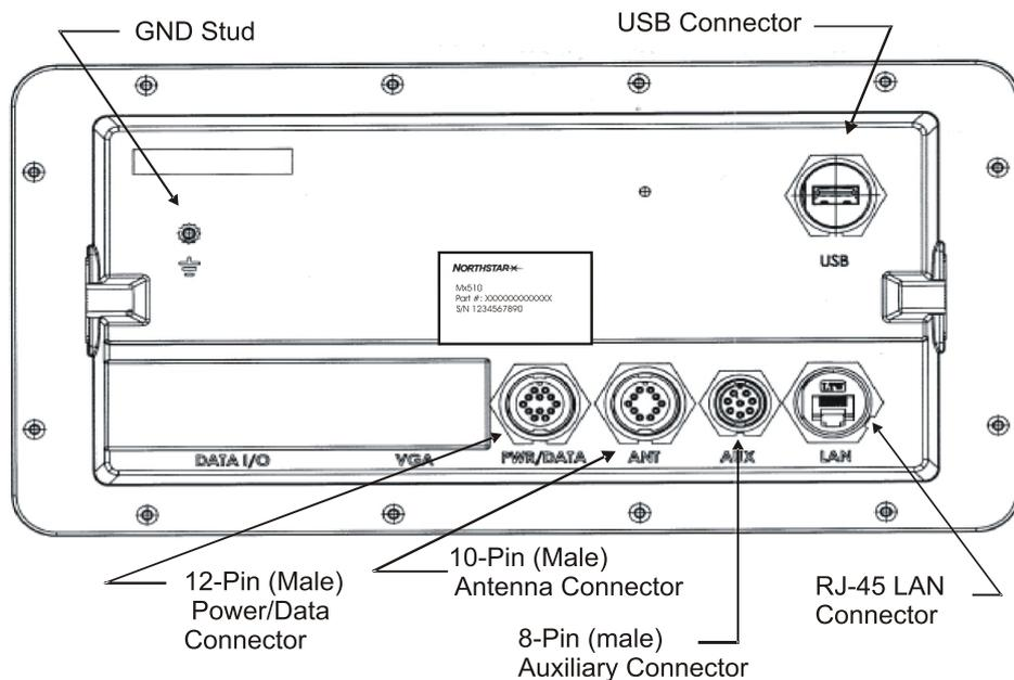
The PWR/DATA cable is standard accessory cable included in the kit. The AUX, LAN and antenna cables are optional items that can be ordered separately. Specify the proper antenna cable length when ordering.
