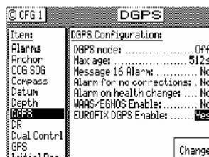
When Loran-C (Raytheon) option is enabled, the MX51x gives the option to accept EUROFIX DGPS corrections instead of the External DGPS corrections under the CFG1/ DGPS Configuration screen.
