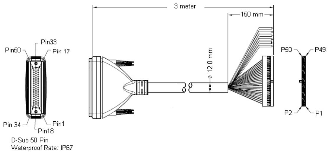
Figure E-5: 50-Pin Cable Assembly (part B)
