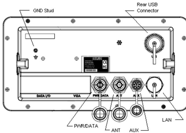
**Figure 5.3 - MX 510 Rear Connector Configuration**
