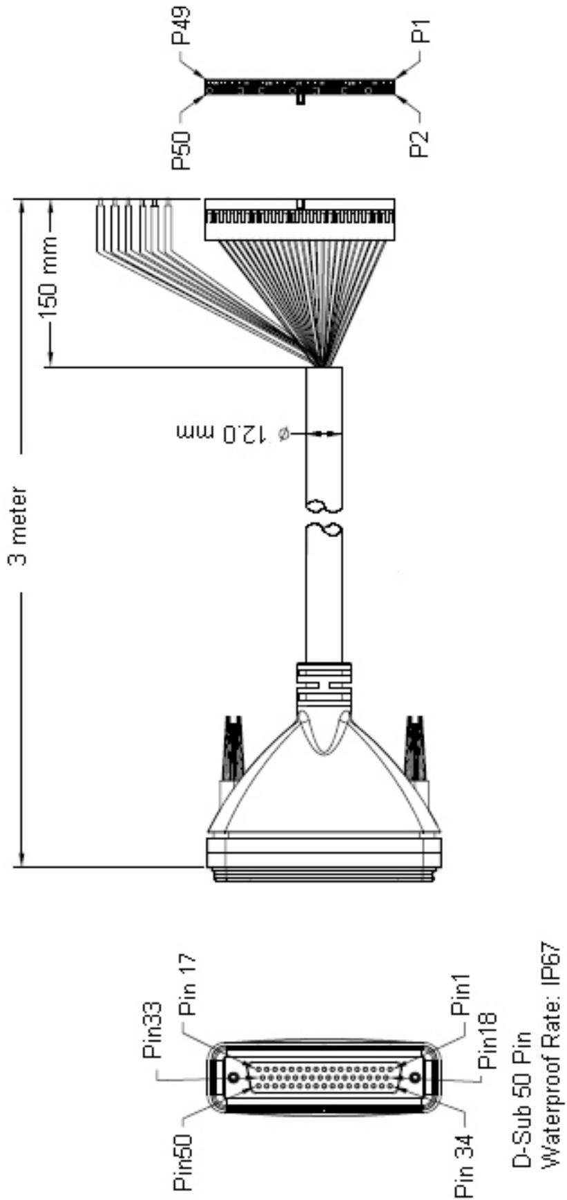
Figure E-4: 50-Pin AIS Cable Assembly
