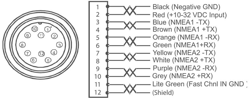
Figure 5.15 Power/Data Cable Diagram
