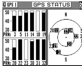
The right window indicates where the satellites are located in the sky relative to your present position. The outer ring represents 0° elevation. The inner ring represents 45° elevation. The center represents 90° elevation and your present position. Under normal conditions, the best satellites to track are usually between 15 and 75 degrees in elevation.
