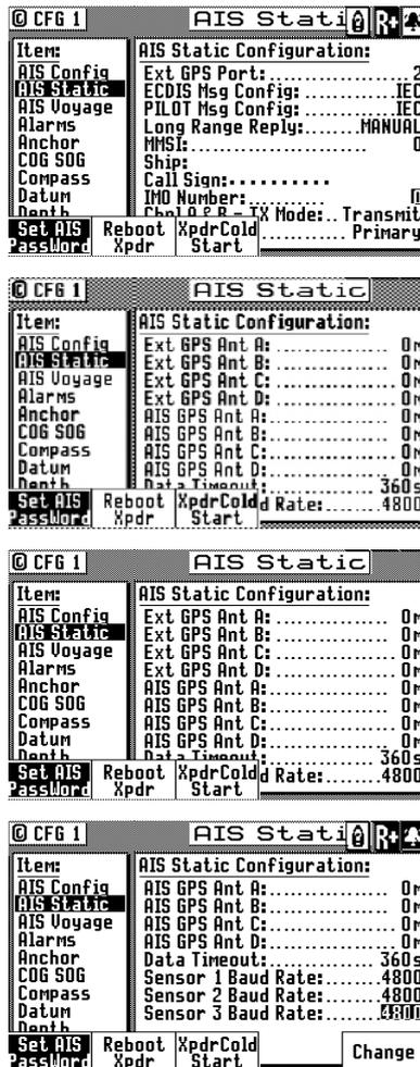
**Note:** A total of 35 lines are available under the AIS Static menu. If only 10 lines are available when you scroll down, the MX512 may not be communicating with the transponder. Verify that the "AIS Connected" value is set to YES and the correct transponder type is selected.
