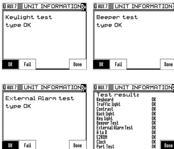
Upon completion of the above tests, a Test Results screen will be displayed. In addition to the visual tests which you witnessed, the CDU also performs background tests on the program memory (*FLASH ROM*), the real-time *Clock*, and the *Serial (NMEA) Ports*. These tests check about 90% of the CDU. The items which it does not check are the GPS and Beacon receivers in the antenna.
