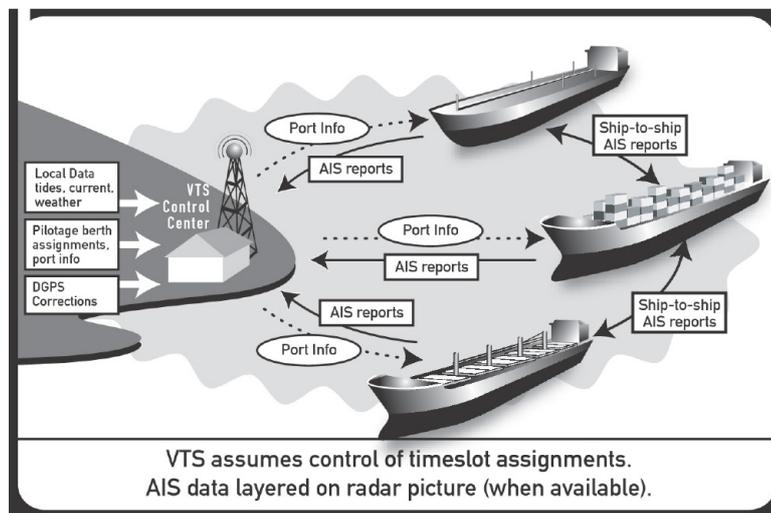
The AIS channels can be used to transmit port data, pilotage, berth assignments,
