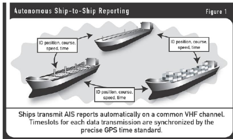
Position and other data are fed automatically from the ship's sensors into the AIS system, where the data is formatted and transmitted in a short data burst on a dedicated VHF channel. When received on the other ships, the data is decoded and displayed for the officer of the watch, who can view AIS reports from all other "Class A" and "Class B" AIS-equipped ships within range in graphic and text format.
