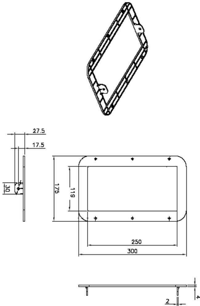
**Figure 5.7 - Optional Flush Mount Frame Dimensions**
