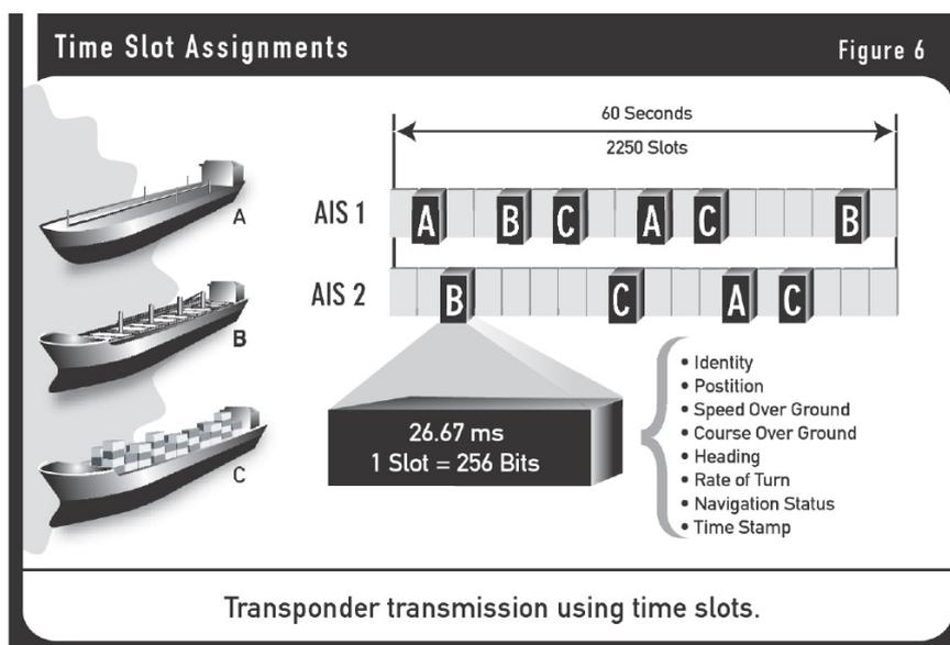
AIS data transmissions utilize a robust 9.6 kbps FM /GMSK (Gaussian Minimum Shift Keying) modulation technique, which is specified in ITU Recommendation M.1371.1. The International Telecommunications Union (ITU) has designated two dedicated frequencies for AIS. They are 161.975 MHz (marine band channel 87B) and 162.025 MHz (channel 88B). In some parts of the world, such as the United States, where these frequencies may not be available for AIS, other channels may be designated.
