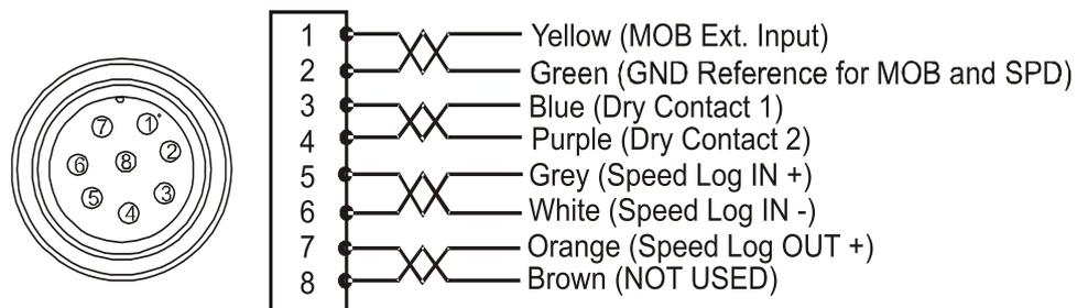
Figure 5.27 - Auxiliary Cable Assembly Diagram
