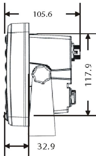
**Figure 5.1- MX51x Display Console Dimensions**
