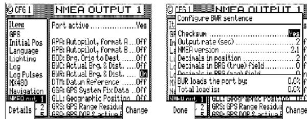
**Decimals In Lat/Lon** - The software allows you to select from 2 to 5 decimal places in records containing position or waypoint information.. The MX51x provides you the flexibility to match the expected input on these devices.
