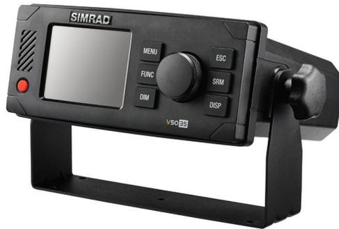
The V5035 consists of a transceiver radio unit, an integrated GPS receiver, a controller unit, and a color 3.5" LCD display with menu keypads. The radio has three receivers -- two TDMA receivers and one DSC receiver. The transmitter alternates its transmission between the two operating TDMA. The controller unit creates and schedules data packets (containing dynamic, static and voyage related data) for transmission based on the IMO performance standard for AIS.
