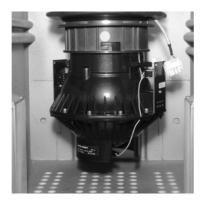
Gently lower the container. The coupling tongues engage into their seats in the bayonet and the container locks in place by its own weight.
