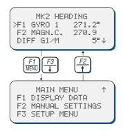
From the normal operational mode, press the **MENU** or the **Down** key to enter the menu mode.
