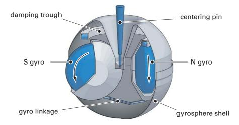
The top of the gyrosphere contains an annular damping trough, half filled with a viscous fluid. The fluid damps azimuthal oscillations of the gyroscope system. The oscillation period is tuned to the Schuler period of 84.4 minutes, so that heading errors during horizontal acceleration due to changes in speed and/or direction are prevented.
