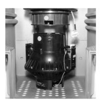
Gently lower the container. The coupling tongues slide down in the grooves of the bayonet and the container is released from the collar.
