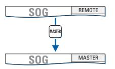
Press the **MASTER** key. Master control is transferred and the mode indication changes from "REMOTE" to "MASTER".
