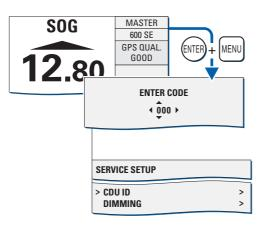
From the normal operational mode, simultaneously press **ENTER** and **MENU** to call up the CDU's local Service Setup menu mode.
