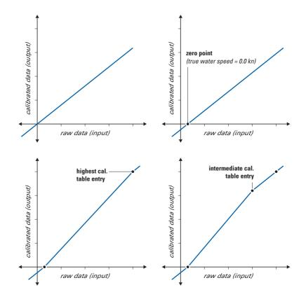
calibration table empty: linear sensor characteristic assumed; display and output = 0.0 kn at raw sensor data value of 0.0 kn
