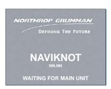
The CDU shows the "waiting for main unit" message for several minutes while the software is downloaded. During the download, the LEDs CR 6, 7 and 22 on the electronics unit PCB will flash in sequence. Upon completion of the download, the system automatically restarts.
