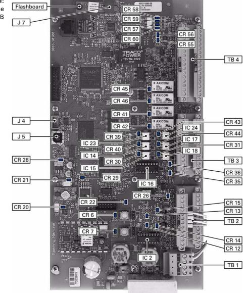
Figure 8-1: location of parts on the processor PCB
