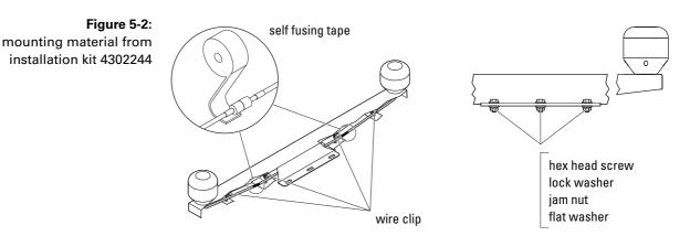
When installing the antenna unit, the cable assembly must be connected to the cables from the bow and stern antenna. After connecting the cables, secure them to the support with the wire clips and seal the cable connections with the self-fusing tape provided.
