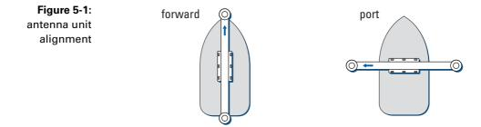
The location of the antenna must provide an unobstructed view of the sky. It should be clear of reflections from masts, out of the path of the radar beam, and out of the range of any object that may shadow or interfere with the reception of GPS signals.
