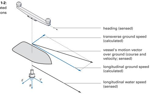
The electronics unit transmits all speed data to receiving external equipment and to the connected CDUs. From the longitudinal ground and water speeds, the electronics unit also calculates the distances travelled and maintains the total and daily mile counters for both the ground and water distances.
