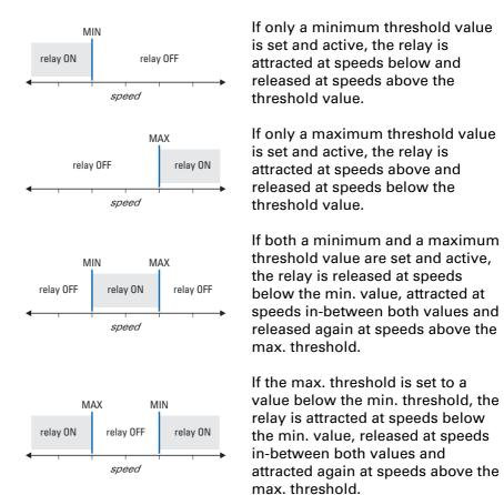
If both threshold values are de-activated or set to exactly the same value, the limit relay function is disabled.
