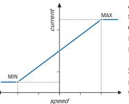
At speeds equal to or below the minimum speed, the output delivers the minimum current; at speeds equal or above the maximum speed, the output delivers the maximum current.
