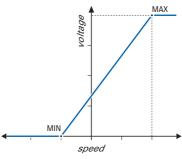
At speeds equal to or below the minimum speed, the output delivers the minimum voltage; at speeds equal or above the maximum speed, the output delivers the maximum voltage.
