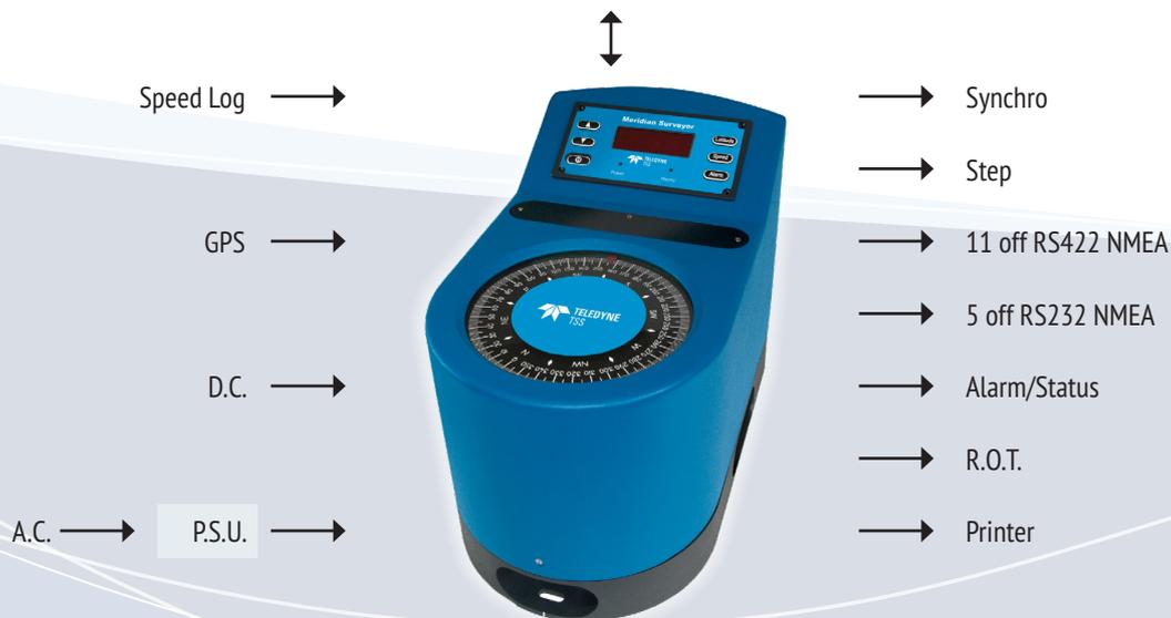
For simple installation the Meridian offers a large array of digital and analogue outputs plus easy to use digital set-up and self-test modes that are activated via the control unit.
