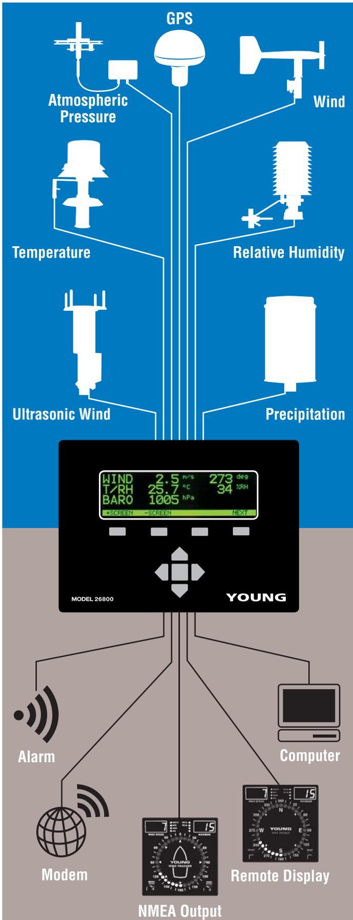
The 26800 is compatible with a wide variety of sensors and accessory devices. Terminals for all functions are readily available on the back panel. Convenient, plug-in terminal blocks simplify wiring and service needs after installation.
