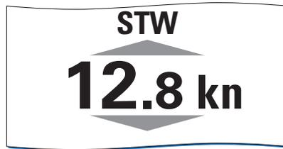
In the normal operational mode, the NAVIKNOT 450 D CDU permanently display the actual speed through the water (STW).
