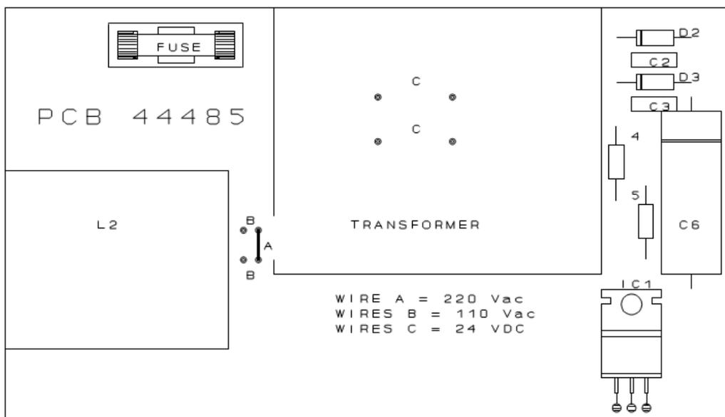
As an option the OMC-138/139 can be delivered for 12 Vdc, If the unit has to be modified to work with 12 Vdc the transformer has to be removed. With the transformer removed it becomes possible to install a DC/DC converter on the location of the transformer. The DC/DC converter converts the 12 Volt supply voltage up to 24 Vdc.
