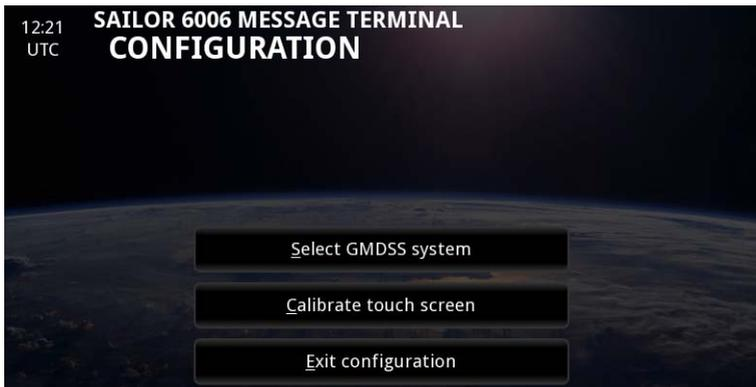
1. "Calibrate touch screen" is only used for Message Terminals with resistive touch screen (early models).
