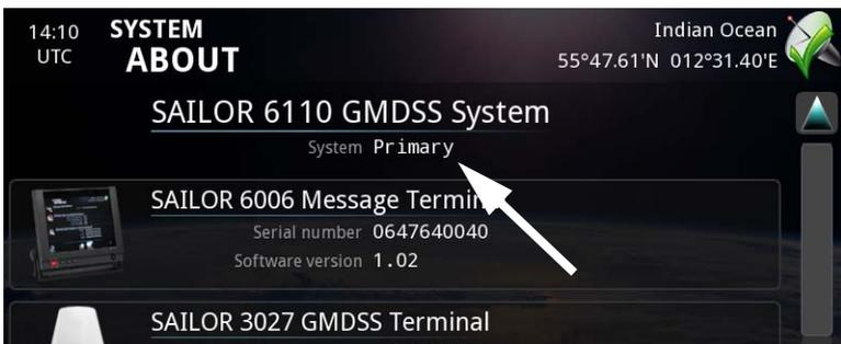
If you have an Alarm Panel in the system, the primary and duplicated systems will appear in the Alarm Panel as Inm-C 1 and Inm-C 2 respectively.
