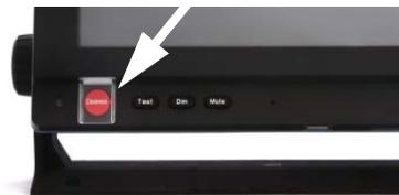
During this time the button light flashes and the buzzer sounds. After 3 seconds the red light goes steady on and the buzzer is silent. The display shows that the message is being sent.
