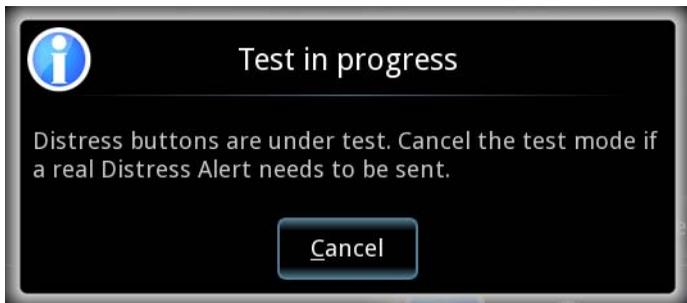
As long as the **Test in progress** window is showing, you can use Distress buttons connected to the system under test, without sending a real Distress Alert.
