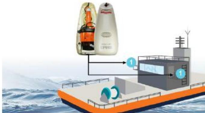
Figure 2: Recommended location of the Tron 40VDR
