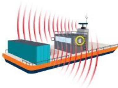
Figure 3: Interference reflected by cargo
