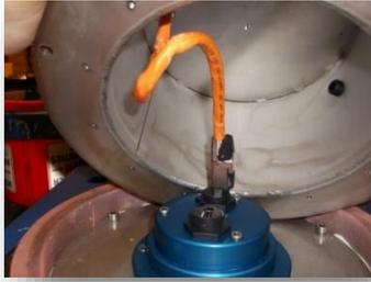
**E)** Once the storage medium and the deckmount are placed upon each other, attach the vulcanized tape around the flanges to ensure water tightness. Stretch around 50cm of vulcanized tape and make sure to wrap it twice around the seam that is between the capsule and the deckmount.
