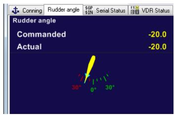
Check that the rudder angle is displayed correctly.
