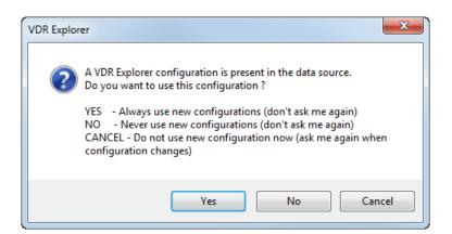
A VDR explorer configuration which matches the VDR data must be uploaded to the VDR when the VDR is installed. This will enable any PC with the VDR Explorer installed to replay data without any configuration work. If this dialog box appears then select, "Yes".
