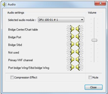
The speaker symbols may be used (by left-clicking on them) for selecting and directing audio channels to the left or right speaker channel on the PC used for replaying.
