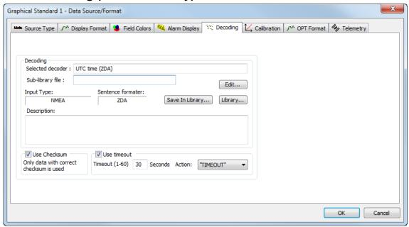
**Edit:** Open the decoder script editor, see section 13.3. The editor is used for creating a new decoder script or for editing the currently selected one. It is strongly recommended that an edited decoder always be given a new name and that the modification is described.
