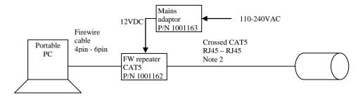
Note 2) if the original cable is attached to the capsule, then use a straight CAT5 cable and a RJ45 coupler.
