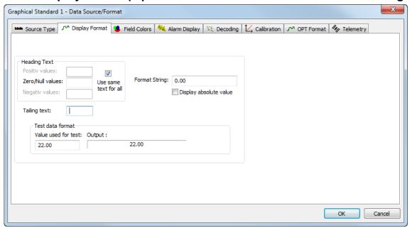
The parameters on this tab are used for formatting analog data or the value output from a decoder.
