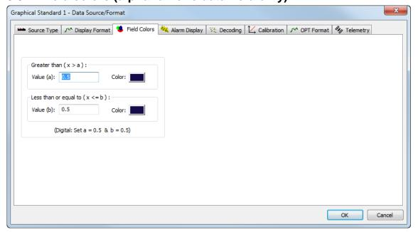
Background color for an alphanumeric data field may be configured to change depending on the displayed value, for example green for indicating SB and red for indication PS.
