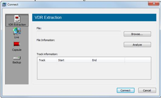
The "Connect" dialog box is used for connecting the VDR Explorer to a data source. Four types of data sources are supported:
