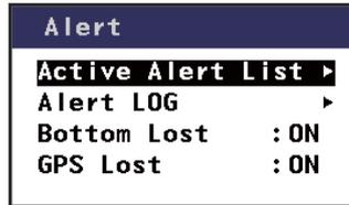
4. Select [Active Alert] list using **▲** or **▼**, then press the **ENT** key.
