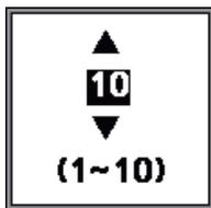
5. Adjust the [TX Rate] using ▲ or ▼, then press the **ENT** key to apply the settings and close the pop-up window. The higher the setting, the higher the rate at which the FE-800 outputs a signal. To keep the default setting (10), press ◀ or the **MENU/ESC** key.
