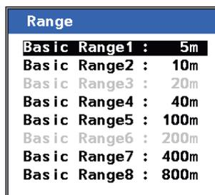
4. Select the basic range scale using ▲ or ▼, then press the **ENT** key. This will open a pop-up window.
