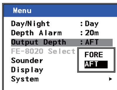
The selected transceiver is highlighted as shown in the figure below.
