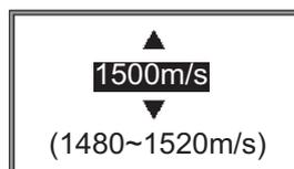
5. Adjust the parameter using ▲ or ▼, then press the **ENT** key to apply the settings and close the pop-up window. To keep the default setting, press ◀ or the **MENU/ESC** key.
