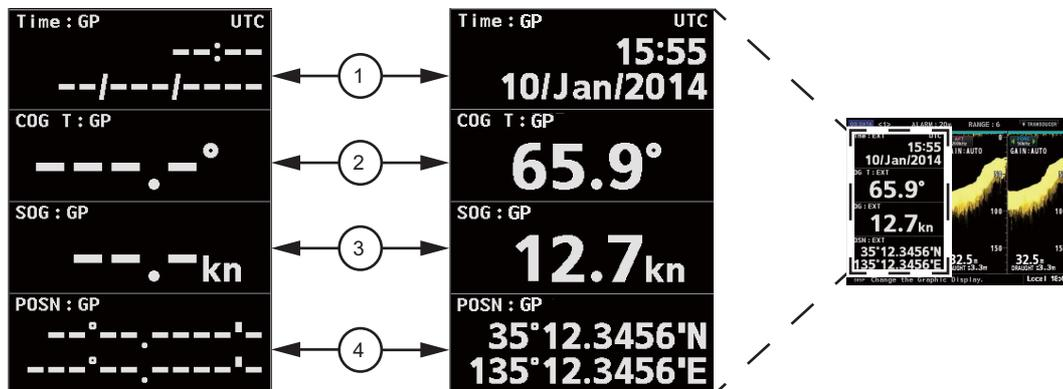
The OS DATA mode requires a connected EPFS device, such as GPS. If there is no device connected, or connection is interrupted, the OS DATA is displayed as shown in the above left figure. The left side of the display shows the OS DATA, the right side of the display shows the current echo readings.
