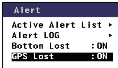
5. Select [ON] to output an alert, select [OFF] to stop alert output.
