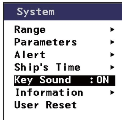
4. Select [ON] to output a sound, select [OFF] to stop sound output.
