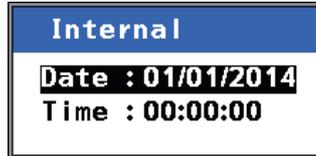
5. Select [Date] or [Time] as appropriate, using ▲ or ▼, then press the **ENT** key.
