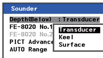
4. Select the location to take the depth reading from, then press **ENT** to apply the settings and close the pop-up window. The available options are [Transducer], [Surface] and [Keel].
