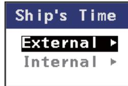
In configurations where the time source is set to [External] and the source signal is lost (for example, the GPS fails), the unit reverts to the internal clock and the time is displayed in yellow.
