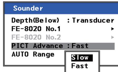
4. Select [FAST] or [SLOW] as appropriate, using ▲ or ▼, then press the **ENT** key.
