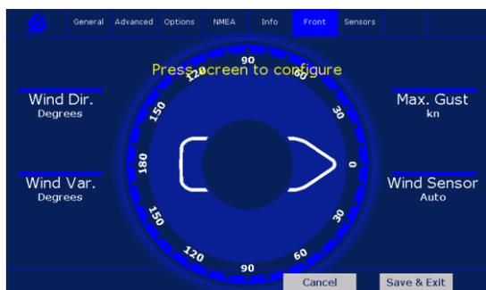
The wind circle & boat can be rotated in steps of 90°. This is useful in case the display is mounted sideways or on the aft.
