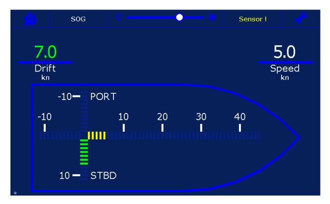
The STW screen shows the speed through water and drift of the vessel.
