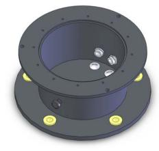
Figure 13-4 - When feeding the cables (through the deck) from the bottom, alternative cable entries may be used by interchanging the cable glands and blind plates.
