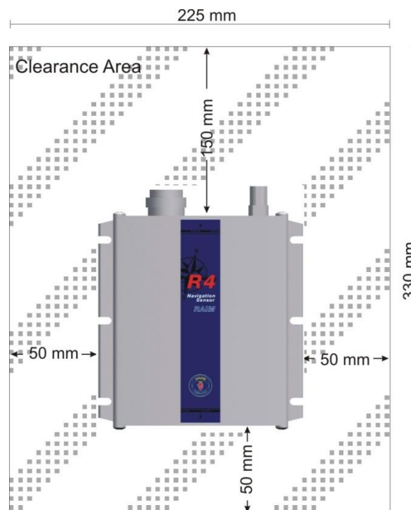
Figure 6 – Clearance Area for R4 Navigation Sensor
