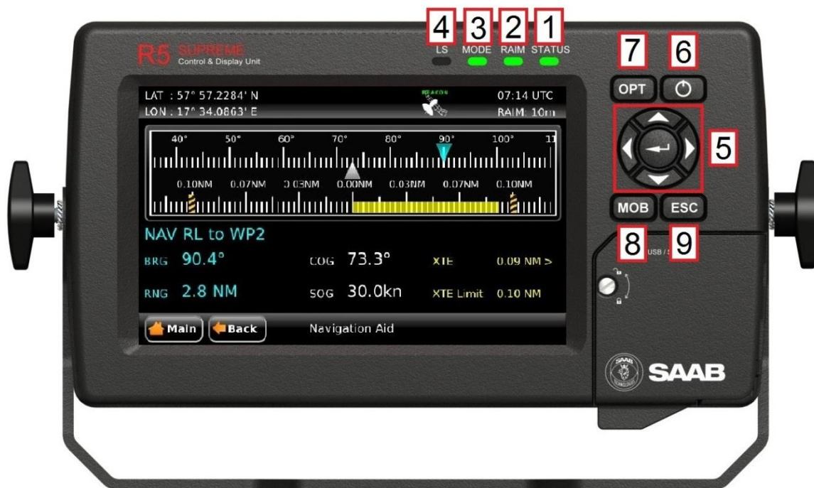
Figure 18 – LEDs and Buttons on CDU
