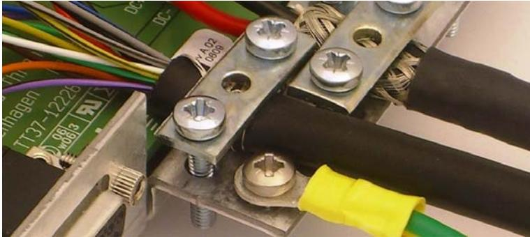
Figure 20 Fixation of the transceiver cable in TT-3616D.
