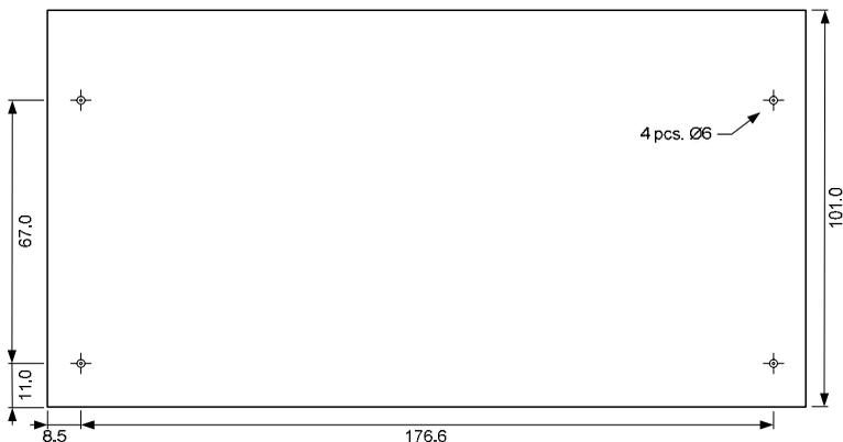
Figure 15 *Drill template. All measures in mm.*
