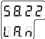
The displayed latitude value is calculated based on the vessel's true bearing and the vessel's actual speed. Refer setting the latitude input source and speed input source, page 53 onwards.
