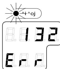
If more than 4 alarms are active, this will be indicated with a dot behind the last number as shown on the figure below. Further alarm codes may then be displayed by pressing the “arrow up” button.
