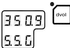
Confirm that the gyro compass's displayed true bearing is according to a known target or astronomical observation.
