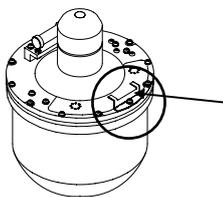
**6** Fasten the screw on the plug holder on the defective Sensitive element.
