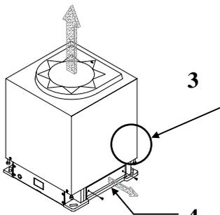
**3** Remove the four screws holding the compass case, and lift the case carefully upwards and away.
