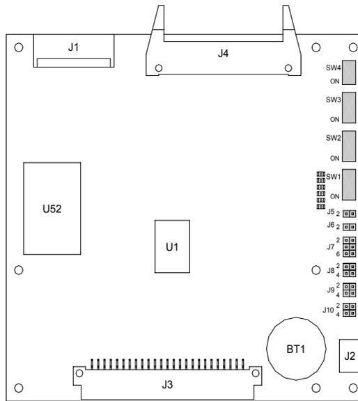
**DIP switch settings on SCC board**
