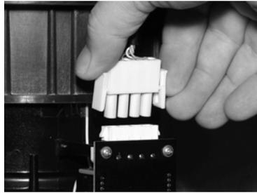
9. Plug the gyrosphere supply and pickoff connector into its socket on the gyrosphere container.
