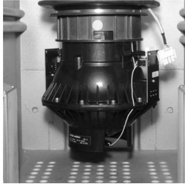
8. Gently lower the container. The coupling tongues engage into their seats in the bayonet and the container locks in place by its own weight.
