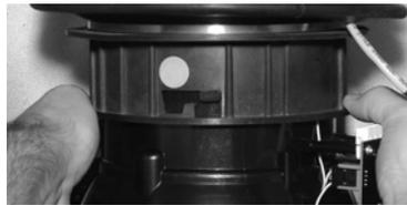
6. While supporting the container with both palms, put the thumbs on the rim of the collar, pull down on it and turn it to the left
