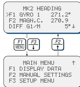
From the normal operational mode, press the **MENU** or the **Down** key to enter the menu mode.
