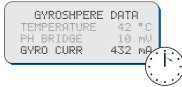
Directly after power-up, the gyrosphere current should not exceed 550 mA. The current will gradually fall while the gyrosphere settles.
