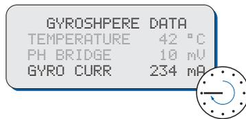
Within 45 minutes after power-up, the gyrosphere current must have dropped below 300 mA.
