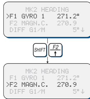
To change the active heading source from the control and display unit
