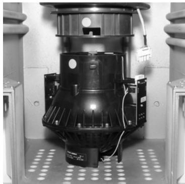
7. Gently lower the container. The coupling tongues slide down in the grooves of the bayonet and the container is released from the collar.
