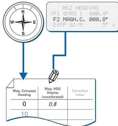
5. While the vessel is turning, compare the indication at the steering magnetic compass with the magnetic heading values shown on the NAVIGAT X MK 2 display.
