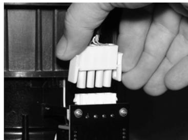
3. Unplug the gyrosphere supply and pickoff connector from its socket on the pickoff PCB.
