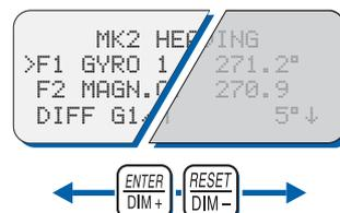
Press the **DIM+** key to increase the illumination brightness. Press the **DIM-** key to reduce the illumination brightness.
