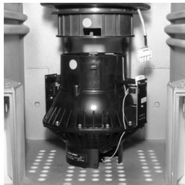
5. Place the gyrosphere container into the compass housing with the largest of the three coupling tongues located directly below the groove in the collar. The tongue is marked by a green dot on the container
