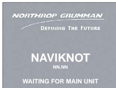
9. The CDU shows the “waiting for main unit” message for several minutes while the software is downloaded. During the download, the LEDs CR 6, 7 and 22 on the electronics unit PCB will flash in sequence. Upon completion of the download, the system automatically restarts.
